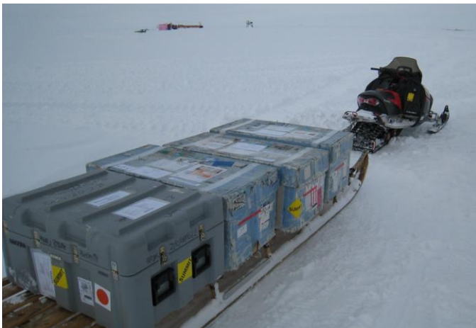
Figure 4 Photo of the BuckEV attached to the sled used to pull scientific equipment to remote testing locations near the NSF's Summit Station in Greenland.
