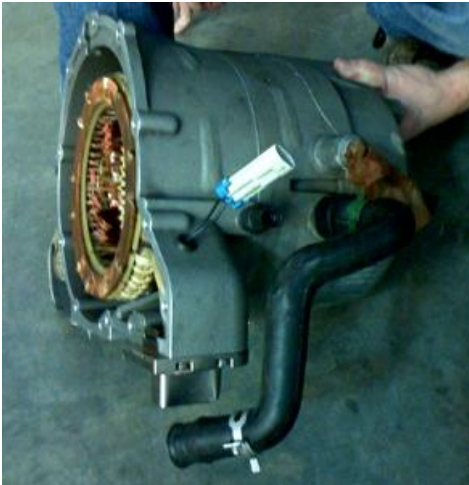
Figure 8 Photograph of the Delphi EV1 copper-bar-rotor AC induction electric motor, with a peak power of 100 kW.
