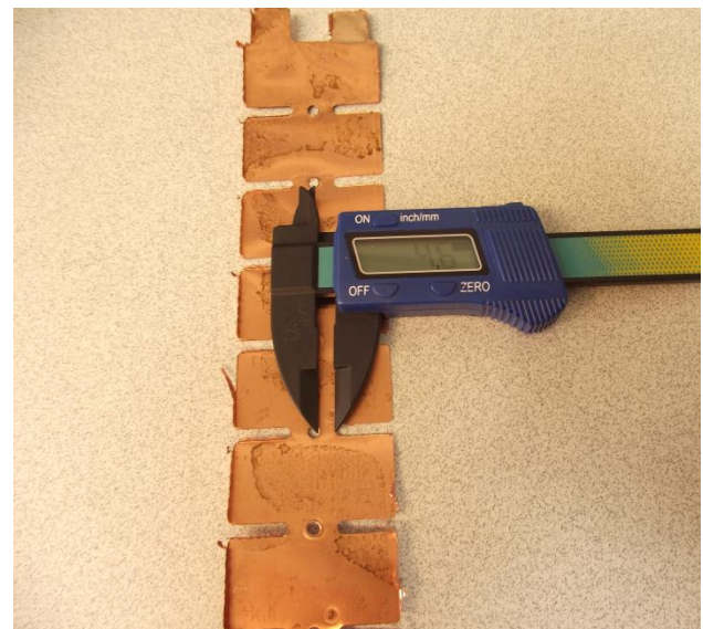
Figure 15 Picture showing the common conductor fuse used to connect the individual cells.
