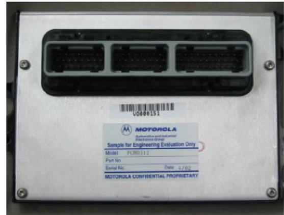
**Figure 17.** Picture of the ECM-0555 powertrain control module
