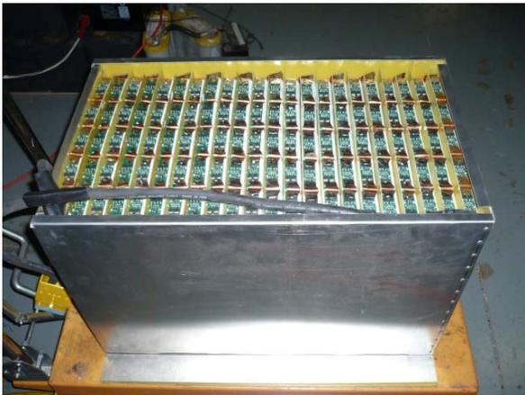
**Figure 16.** Picture of a fully assembled battery pack just before the cover is installed [14].
