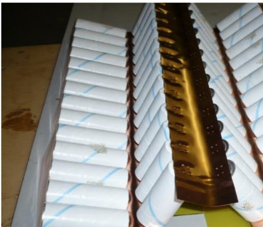
**Figure 14.** Picture showing the common conductor created at each cell interconnect node [14].
