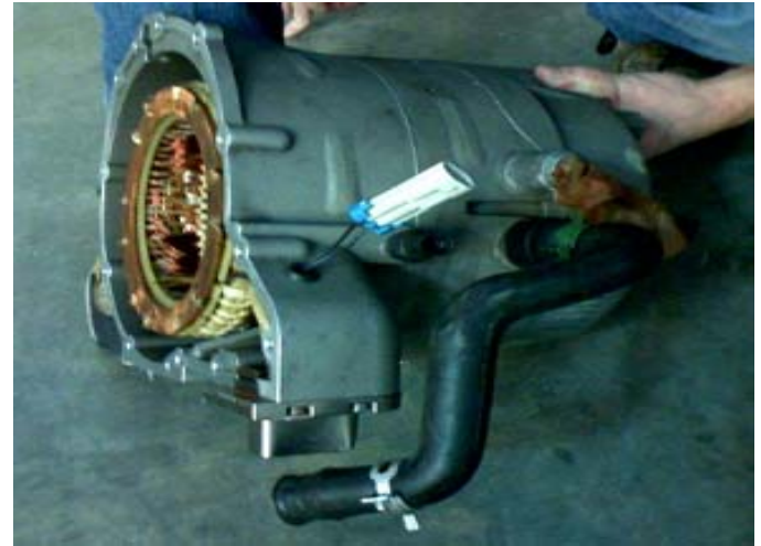
Figure 7 Photograph of the Delphi EV1 copper-bar-rotor AC induction electric motor, with a peak power of 100 kW. The transaxle used in the GM EV1 was removed and replaced with a student-designed endplate (not shown).
