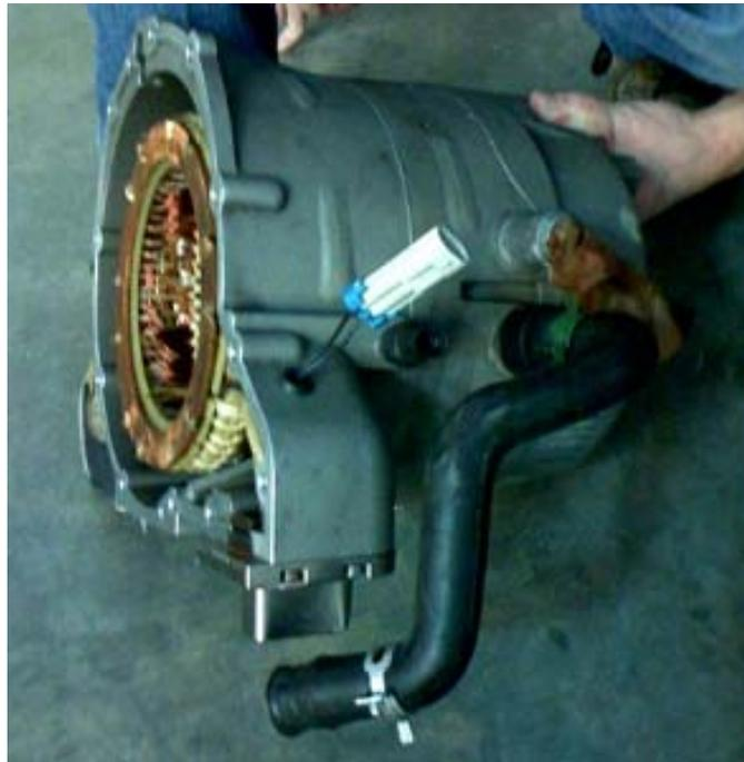
**Figure 4** Photograph of the Delphi EV1 copper-bar-rotor AC induction electric motor, with a peak power of 110 kW. The transaxle used in the GM EV1 was removed and replaced with a student-designed endplate (not shown).
