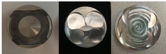
Figure 11: Pictured from left to right: stock Rotax piston, unmodified Honda piston, and machined Honda piston with two tier piston bowl design to improve mixing in combustion chamber
