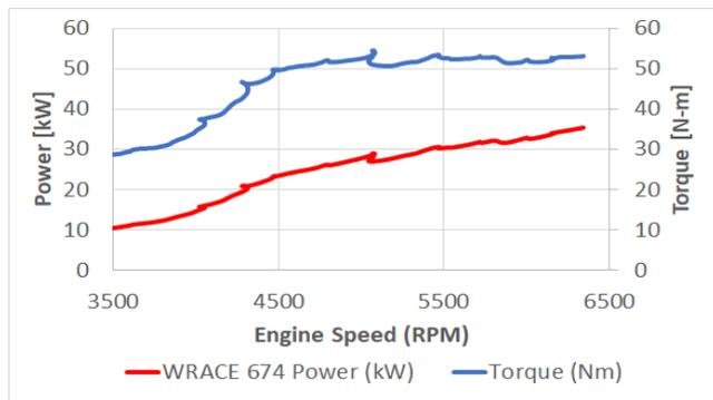
Figure 12: Experimental dynamometer torque and power curves for the optimized WRACE 674 engine
