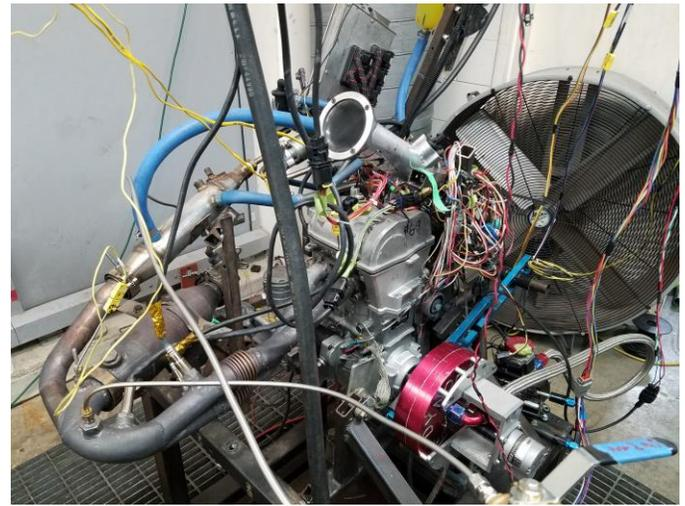
Figure 17: Dynamometer testing stand used for calibrations
