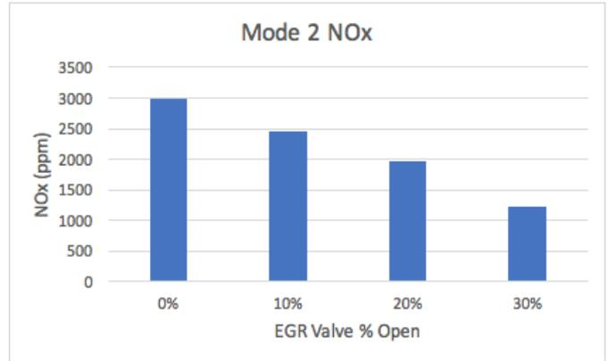
Figure 20: Recorded NO<sub>x</sub> emissions in the team’s estimated Mode 2 at various EGR percentages, recorded while running non-oxygenated 91 octane fuel
