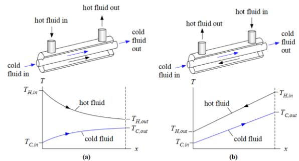
Figure 3: Operational characteristics of counterflow and parallel flow heat exchangers [1]
