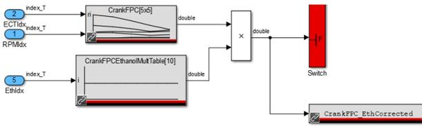
Figure 4: Ethanol based crank fueling multiplier code block
