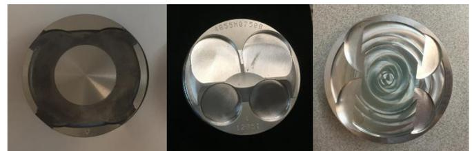
Figure 13: Pictured from left to right: stock Rotax piston, unmodified Honda piston, and machined Honda piston with two tier piston bowl design to improve mixing in combustion chamber
