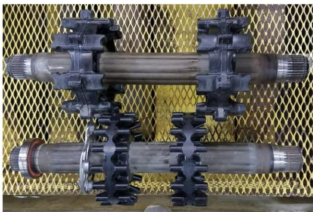
Figure 22: Ski Doo’s standard drive is the top drive pictured above, with the Silent Drive below it
