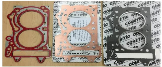
Figure 14: Pictured from left to right: stock Rotax head gasket, copper head gasket, and composite fiber head gasket with fire ring
