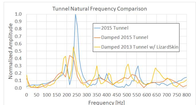
Figure 1: Normalized tunnel frequency amplitude comparison of damped and undamped 2015 chassis and dampened 2013 chassis
