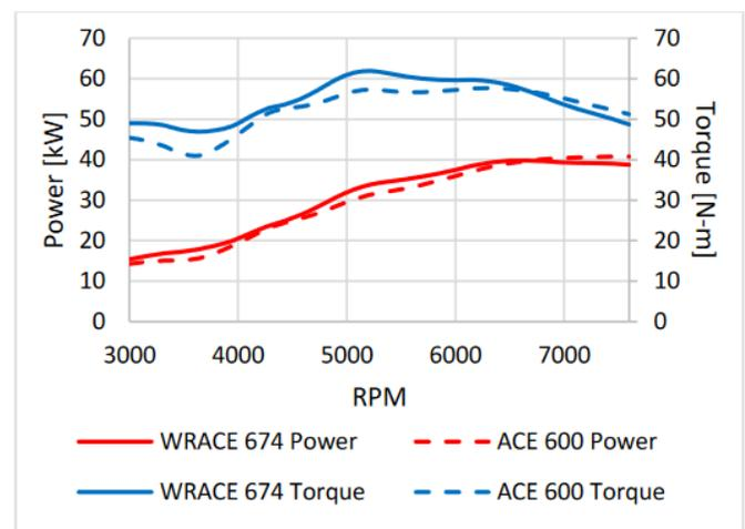
Figure 11: Torque and power curves for the stock ACE 600 and optimized WRACE 674 engines simulated with a Ricardo Wave model
