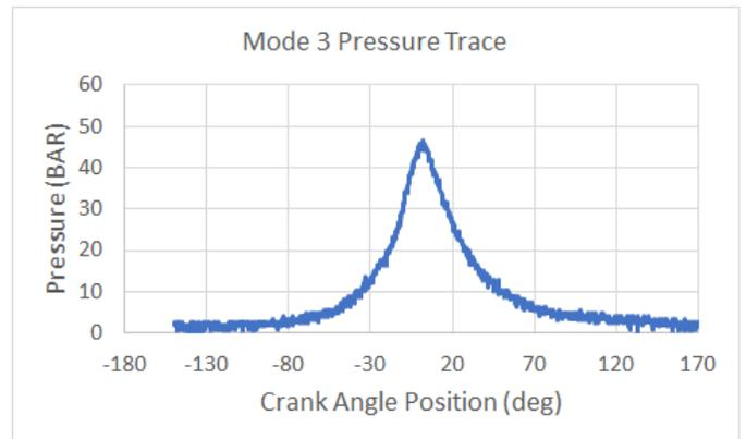
Figure 18: In-cylinder pressure at emissions mode 3
