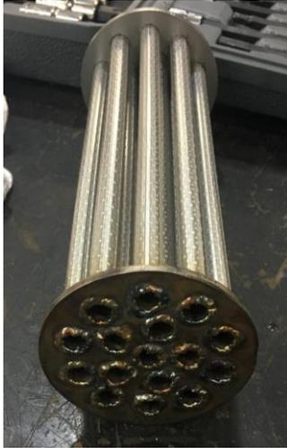
Figure 19: The sixteen tubes of the cooler were spaced to maximize the amount of turbulence in the cooler resulting in the highest amount of heat transfer out to the engine coolant
