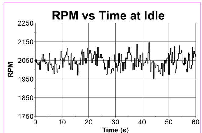
Figure 7: New spark PD controlled idle engine speed in RPM over 60 s run time
