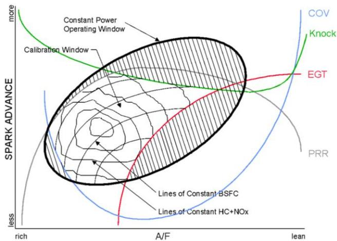
Figure 16: Graph of typical calibration window [2]
