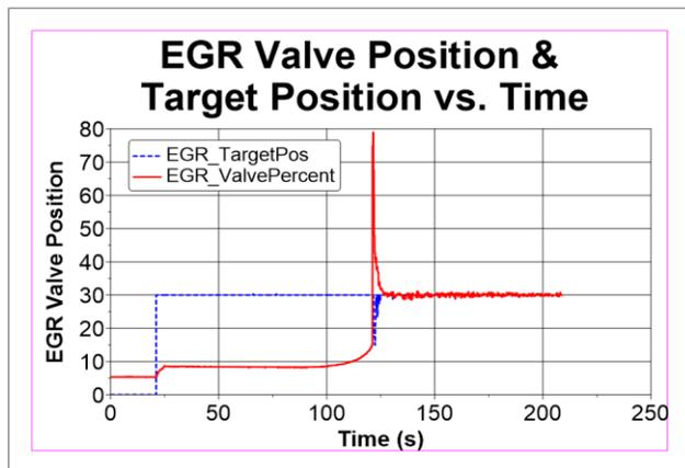
Figure 9: EGR Valve Position and Target Position while idling after a cold start
