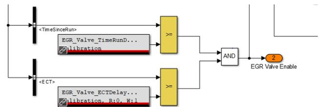
Figure 10: New branch of Simulink engine code containing ECT based EGR valve delay
