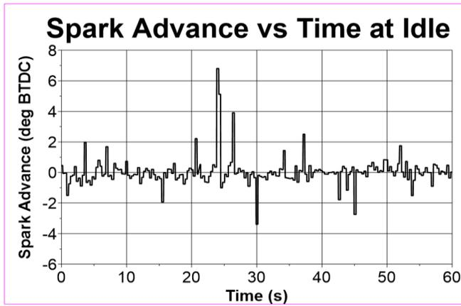
Figure 8: Spark Advance response to rapid EGR Valve Movement over 60s run time
