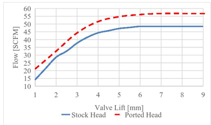
Figure 15: The exhaust ports of the ported head compared to the stock head. The ported head shows flow improvement across the valve lift profile
