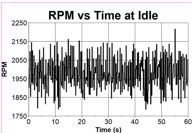
Figure 5: Engine Speed (RPM) at idle over 60 s run time
