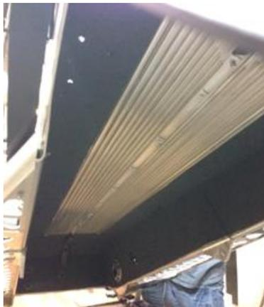
Figure 2: View of tunnel underside lined with Lizard Skin material
