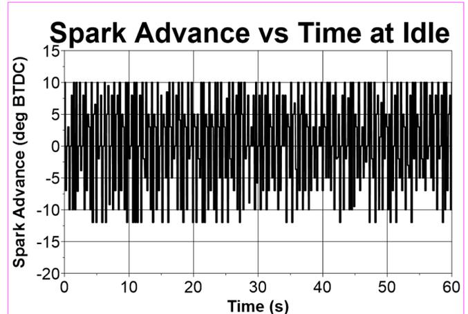
Figure 6: Spark Advance (degrees BTDC) at idle over 60 s run time
