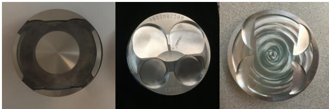
Figure 4. From left to right: stock Rotax piston, unmodified Honda piston, and machined Honda piston with two tier piston bowl design to improve mixing in combustion chamber.
