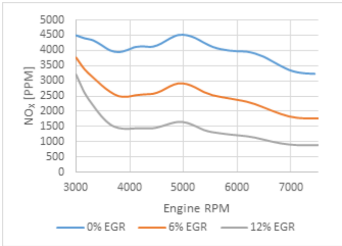
Figure 14. Simulated engine out NO x of the WRACE 674 using volumetric percentages 0%, 6%, and 12% EGR.
