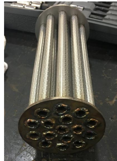
Figure 13. The 16 tubes of the cooler were spaced to maximize the amount of turbulence in the cooler resulting in the highest amount of heat transfer out to the engine coolant.
