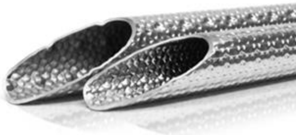
Figure 11. The enhanced surface of the tubes manufactured by Vipertex. The increased roughness of the walls disrupts the boundary layer creating turbulent flow, which increases the amount of heat transfer from the recirculated exhaust gas to the engine coolant.
