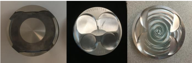
Figure 3. From left to right: stock Rotax piston, unmodified Honda piston, and machined Honda piston with two tier piston bowl design to improve mixing in combustion chamber.
