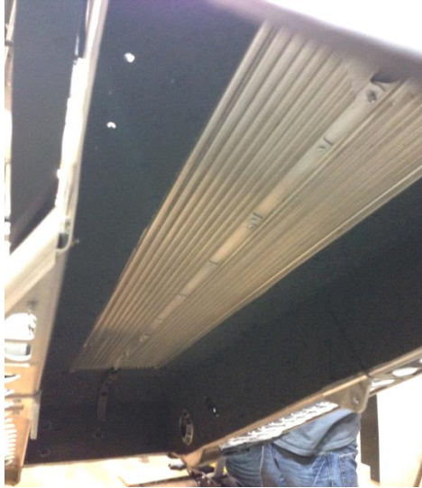
Figure 15. View of tunnel underside lined with Lizard Skin material.
