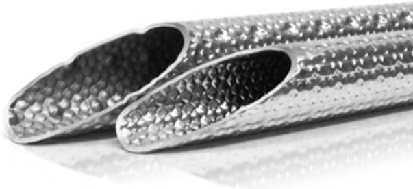
Figure 8. The enhanced surface of the tubes manufactured by Vipertex. The increased roughness of the walls disrupts the boundary layer creating turbulent flow, which increases the amount of heat transfer from the recirculated exhaust gas to the engine coolant.
