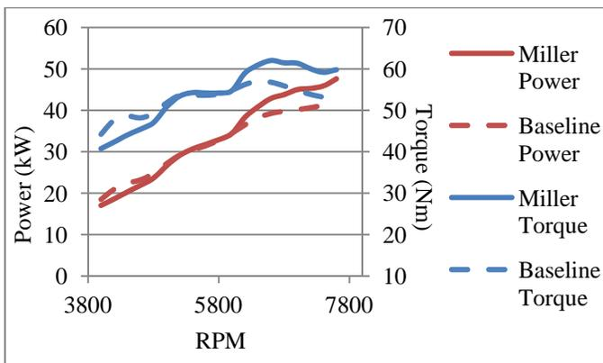
**Figure 12. Torque and horsepower curves for the baseline and optimized Miller cycle engines.**
