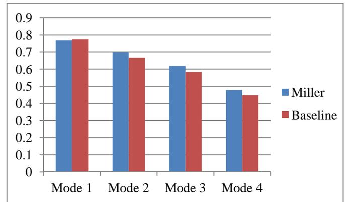
**Figure 10. Fraction of gross indicated work converted to brake work at each mode.**
