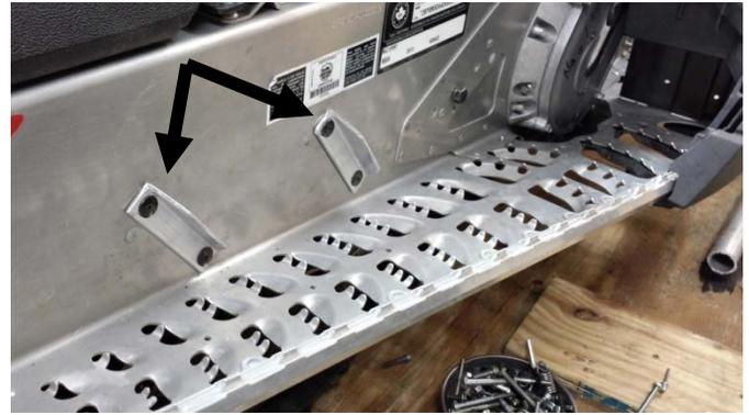
**Figure 22. Tunnel stiffening brackets.**
