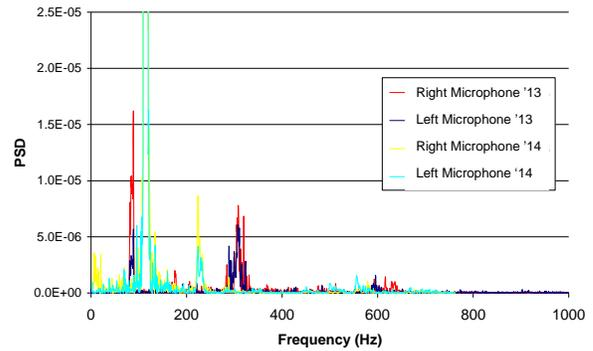
**Figure 18. Spectral sound density of past UW-Madison CSC entries to determine typical sources of noise from a snowmobile.**
