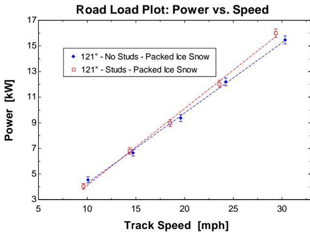
**Figure 23.** Plot showing the effect adding studs had on the power required at various speeds.
