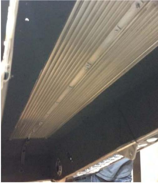
**Figure 20. View of tunnel underside lined with Lizard Skin material.**
