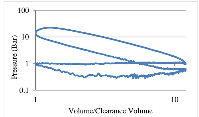
**Figure 13. Pressure-Volume diagram of physical engine during mode 4 operation.**
