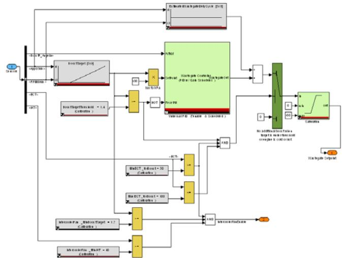
**Figure 4. Image of control strategy Simulink Model for electronic turbo boost control.**
