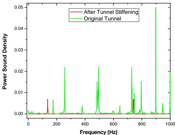
**Figure 21. Chassis frequency spectrum before and after tunnel stiffeners.**
