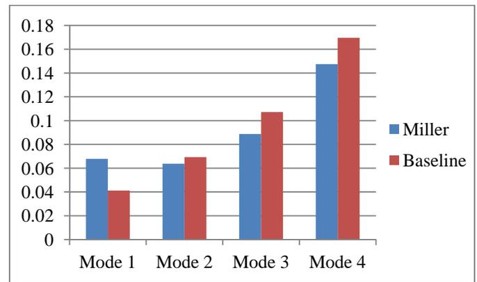
**Figure 9. Modeled fraction of gross indicated work lost to pumping work at each mode.**
