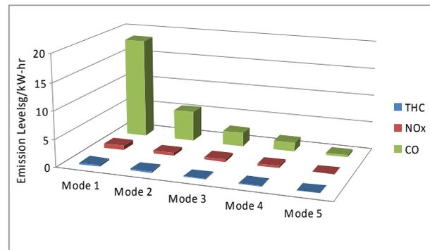
**Figure 17. Emissions breakdown of modes 1 through 5 for the 2014 CSC entry.**
