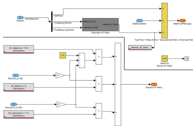
**Figure 14. SimuLink block diagram for flex-fuel and iso-butanol engine control strategy.**
