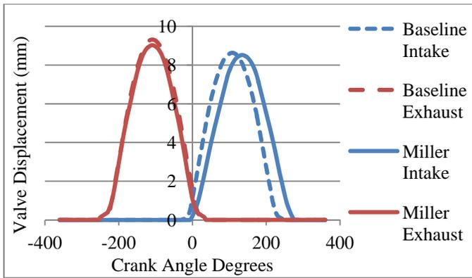
**Figure 7. A comparison of baseline and Miller cycle valve lift profile used for modeling comparisons.**
