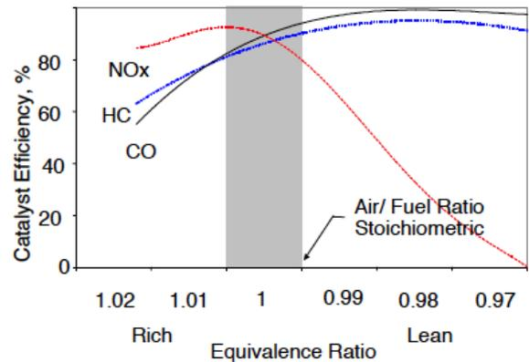
**Figure 15. Shows the NO<sub>x</sub>, CO, and HC conversion efficiency for a three-way catalytic converter as a function of exhaust gas air/fuel ratio operating on gasoline (Adapted from [6]).**
