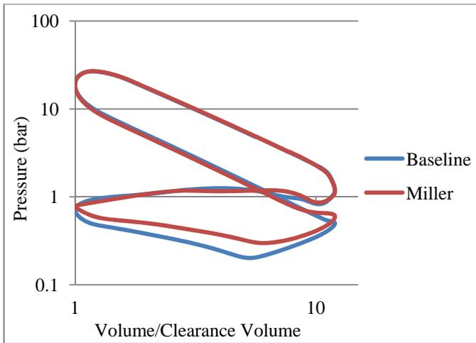
**Figure 11. Pressure-Volume diagram of baseline and optimized Miller cycle engines at Mode 4.**
