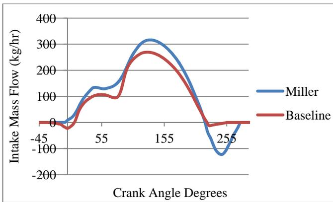
**Figure 8. Modeled intake valve mass flow as a function of crank angle.**
