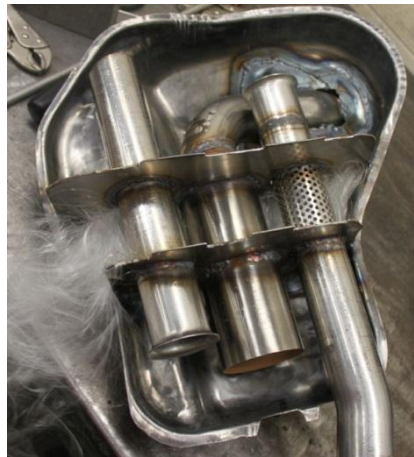
Figure 12: Three-chamber catalytic muffler designed for the Bucky Rush during fabrication.
