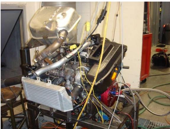
**Figure 10:** Picture of the Weber MPE 750 equipped with the custom camshaft operating on Madison dynamometer stand.
