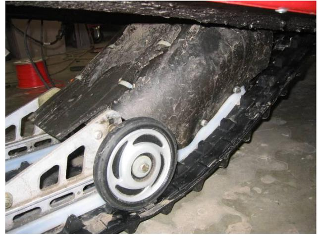
**Figure 15:** Picture of the drive paddle sound dampener installed on front suspension arm.
