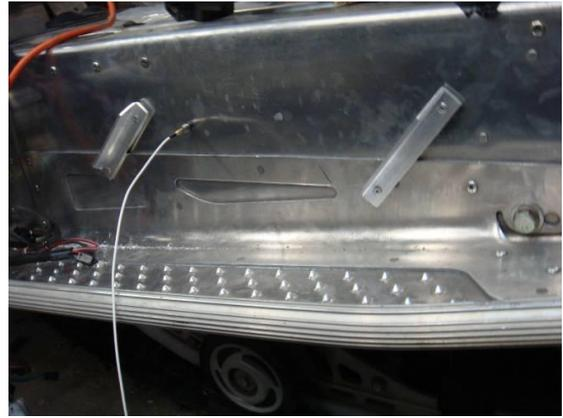
**Figure 18:** Picture of tunnel resonance being tested with tunnel stiffening ribs installed.
