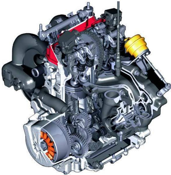
**Figure 4:** Model of the personal watercraft version of the Weber AG MPE 750 engine.
