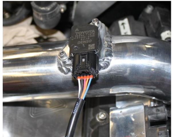
**Figure 7:** Picture of the flex fuel sensor and post-turbo mass airflow sensor to determine desired fueling rate.
