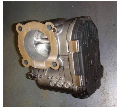
**Figure 6:** Picture of the Bosch electronic throttle body utilized on the Bucky CFS.
