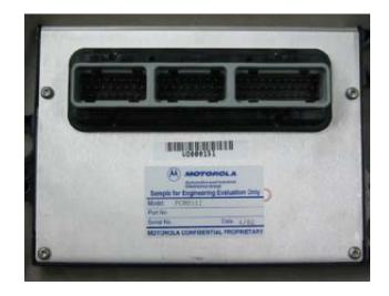
**Figure 6:** Picture of the Motorola MPC555 powertrain control module.
