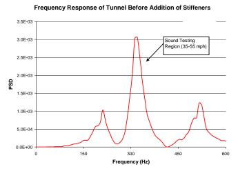
**Figure 19:** Frequency response of tunnel before adding tunnel stiffeners.
