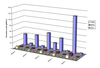
**Figure 10:** Emissions reduction for the FS engine operating on gasoline. The raw engine emissions are on the left side of each mode.
