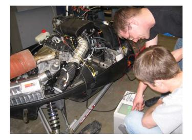
**Figure 7**: Picture of the students huddling around an oscilloscope calibrating the new E85 injectors.
