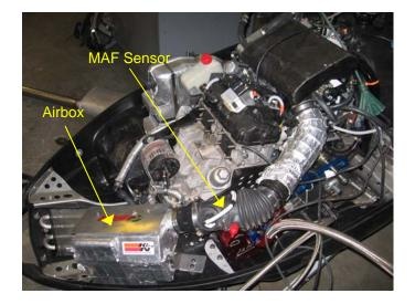
**Figure 3:** Air box construction and location. Note the mass air flow sensor used for engine calibration.
