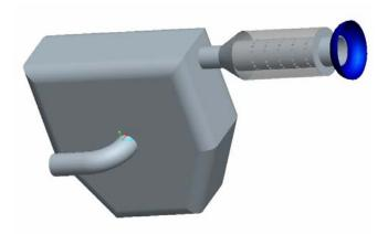
**Figure 13:** The second stage of the muffler system is consists of a high frequency diffuser inline with an Arctic Cat box muffler.
