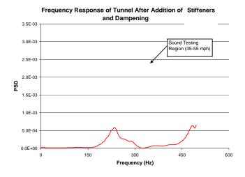
**Figure 21:** Frequency response of the tunnel after adding tunnel stiffeners.
