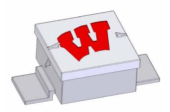
**Figure 23:** Image of the Solidworks model of battery box assembly.
