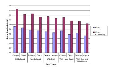
**Figure 18:** Graphs of pass-by sound testing results. The 2007 exhaust is about 1 db quieter than 2006.
