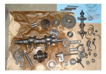
**Figure 5:** Picture of the disassembled engine components prior to the anti-friction coating process.
