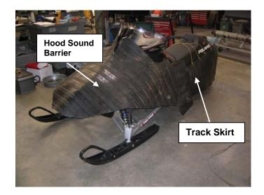
**Figure 17:** Rubber mats were used to isolate sound emissions from targeted components. In this way, the relative contribution of each component to the overall A-weighted sound level could be found.
