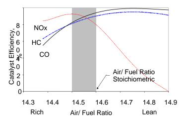
**Figure 8:** The NOx, CO, and HC conversion efficiency for a three-way catalytic converter as a function of exhaust gas air/fuel ratio operating on gasoline (Adapted from [10]).
