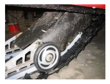
**Figure 16:** Drive paddle sound dampener installed on front suspension arm.
