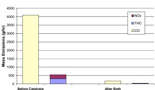
Reduction of Exhaust Gas Emissions Through the Dual Stage Catalyst System (Mode 1, 100% Load)
