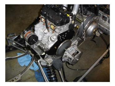
**Figure 2:** Clutch-side engine mounting bracket during fabrication phase.
