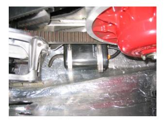
**Figure 11:** The evaporative emissions system on the Bucky Classic 750 reduces hydrocarbon emissions due to thermal cycling of vapors in the fuel tank, a major source of unburned hydrocarbon emissions.
