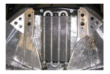
**Figure 4:** Picture of the oil cooler mounting system designed to efficiently cool the FS engine.
