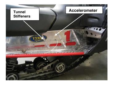
**Figure 20:** Tunnel stiffening angle brackets with accelerometer attached.
