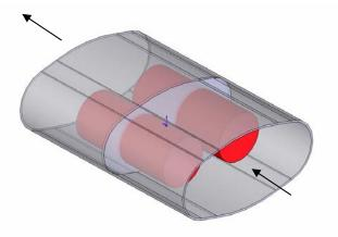
**Figure 12:** Soildworks model of a catalyst expansion chamber.
