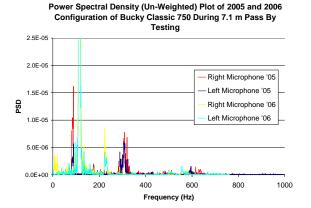
**Figure 14:** Spectral sound density of UW-Madison 2005 and 2006 CSC entries. Testing was performed Feb 25, 2005 and March 1, 2006.
