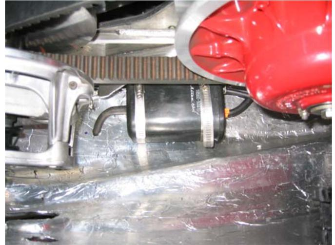
**Figure 10:** The evaporative emissions system on the Bucky Classic 750 reduces hydrocarbon emissions due to thermal cycling of vapors in the fuel tank, a major source of unburned hydrocarbon emissions.
