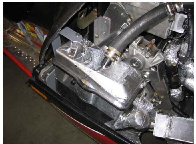
**Figure 5:** Image of the oil reservoir mounted in the Bucky Classic 750.
