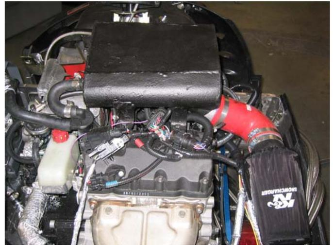
**Figure 4:** Image of the custom air box mounted over the engine.
