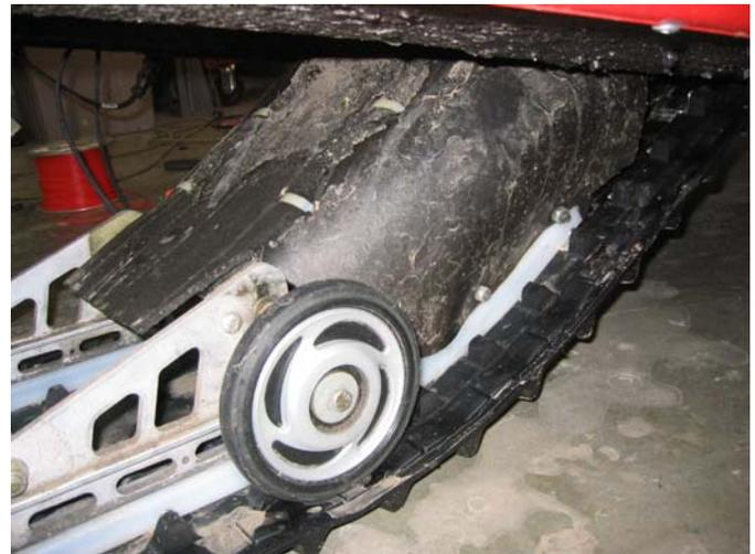
**Figure 15:** Drive paddle sound dampener installed on front suspension arm.
