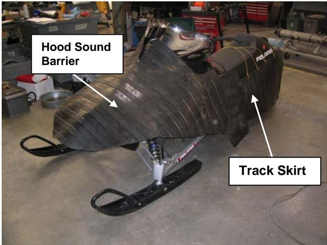
**Figure 16:** Rubber mats were used to isolate sound emissions from targeted components. In this way, the relative contribution of each component to the overall A-weighted sound level could be found.
