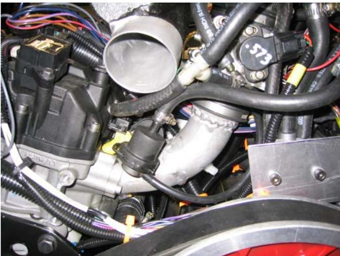
**Figure 3:** Image of custom air induction system used to integrate the stock throttle bodies.
