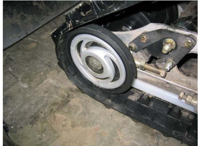
**Figure 14:** Arctic Cat Silent Track installed in the Bucky Classic 750.
