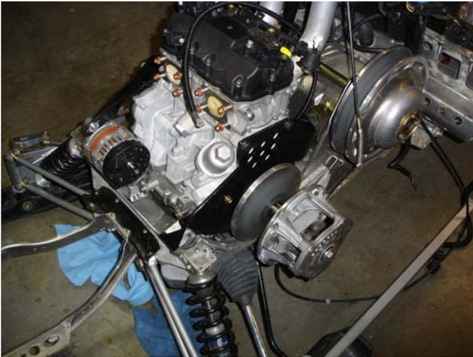
**Figure 2:** Image of the Clutch-side engine mounting bracket during the fabrication phase.
