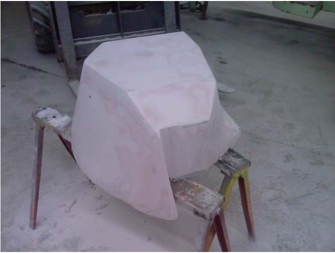
Figure 3 Fabrication of Mold Plug for Side Panel
