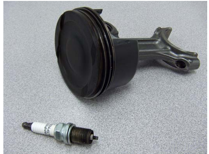
Figure 21. Piston and Spark Plug from Damaged Engine.
