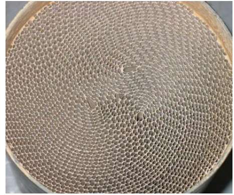
Figure 17. Catalytic Converter Cross Sectional View
