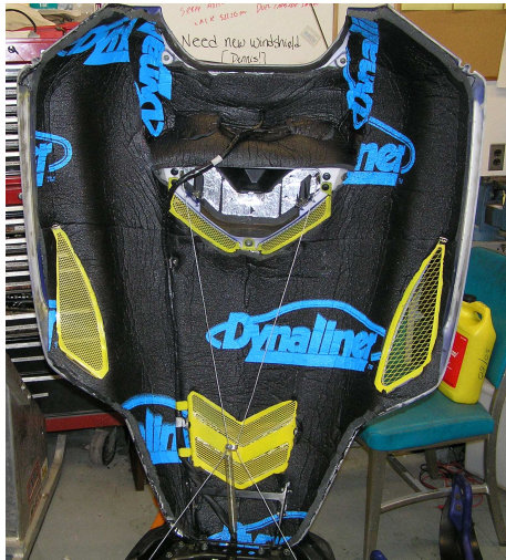
Figure 18. Dynamat noise absorption material underneath the hood.
