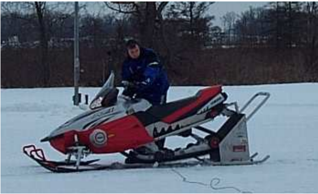
Figure 9. Acoustic engine sweep test
