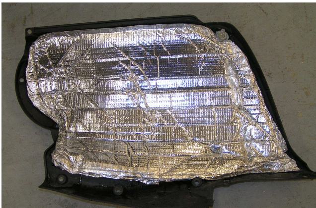
Figure 19. Hoodliner noise absorbing material used in the belly pans that is also water and oil resistant.
