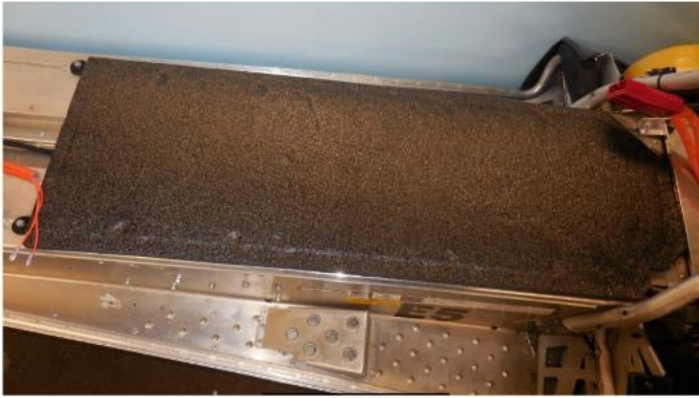
Figure 6: Polyethylene dampening pad
