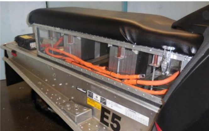
Figure 7: Side view of the battery enclosure/seat
