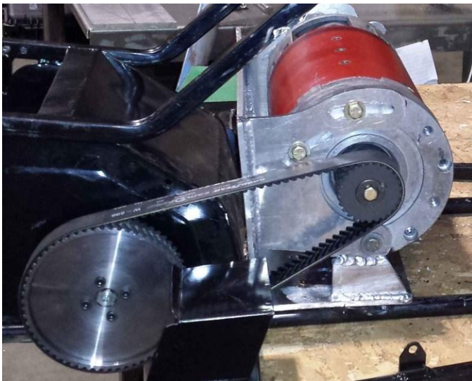
Figure 5. Goodyear Eagle NRG Syncho system mounted on the Snowmobile. The WarP7 motor is painted red on the right-hand side of the picture. The gear ratio takes advantage of running the motor at higher speeds. Some of the material in the stock bottom gear was removed for fabrication and weight purposes.
