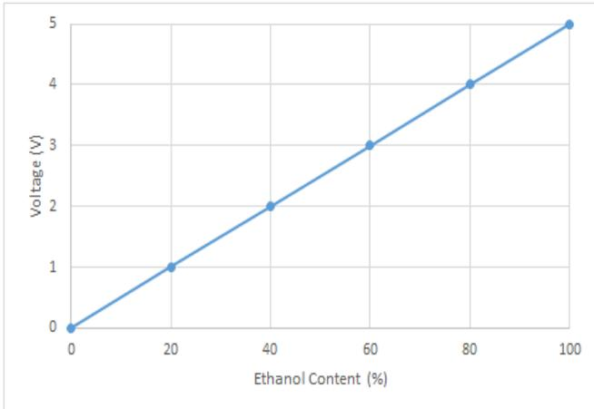
Figure 7: Equating ethanol percentage to output voltage.
