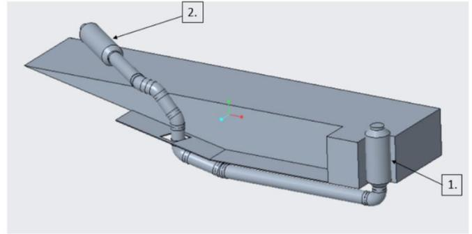
Figure 6. The full assembly of our redesigned exhaust components. At (1) the exhaust flows into the catalytic converter after passing through the stock expansion chamber. After leaving the catalytic converter the piping is run to the back of the snowmobile to the area behind the driver seat and is run to the muffler. At (2) exhaust gas enters the muffler and then exits into the air.
