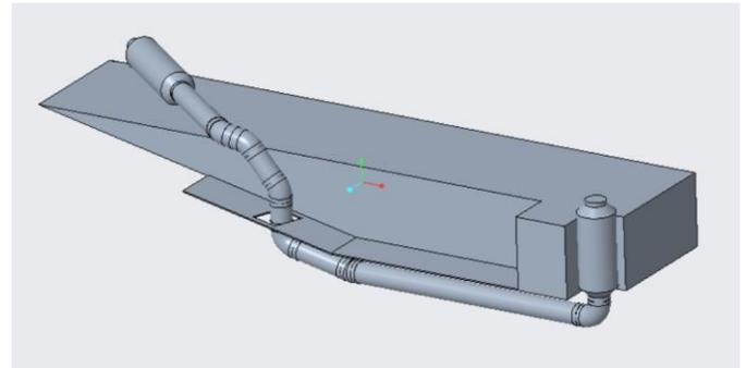
Figure 5: CREO model of the newly designed exhaust system.
