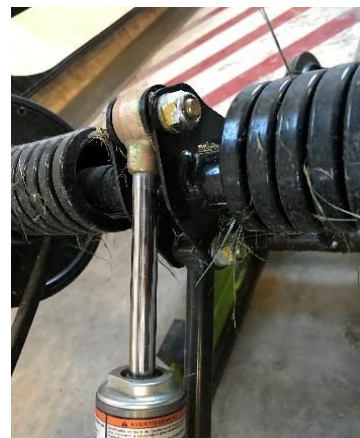
Figure 19: Mounting Location (nut and bolt) for 3D Printed Support Arm
