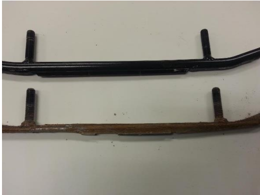
Figure 4. Top: new Trail Blazer IV ski carbides. Below: Worn stock ski carbides.
