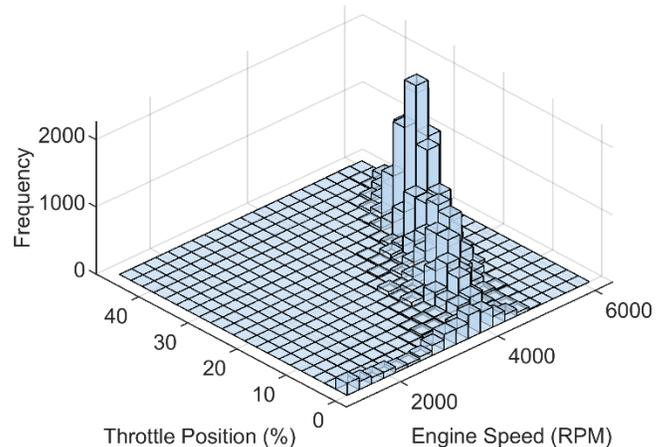
Figure 2. Histogram of engine operation during trail riding similar to the CSC endurance event.
