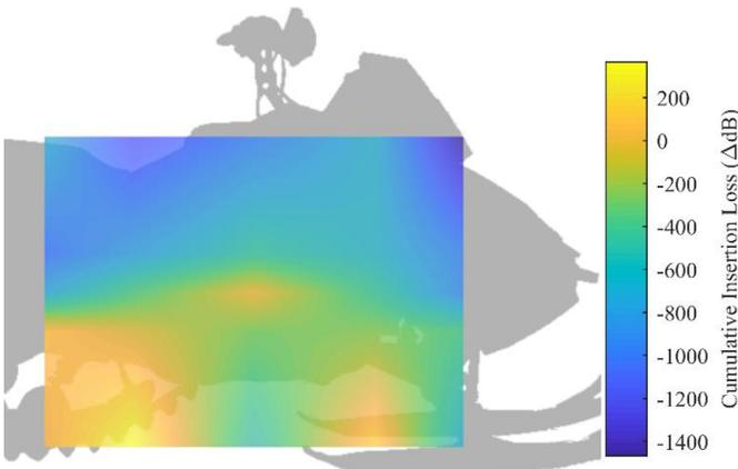
Figure 14. Noise vectoring results from the exhaust side of the snowmobile.
