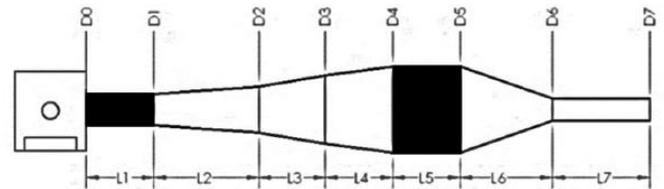
Figure 9. Typical geometry of a tuned pipe. Sections shown in black were extended by the UICSC team.
