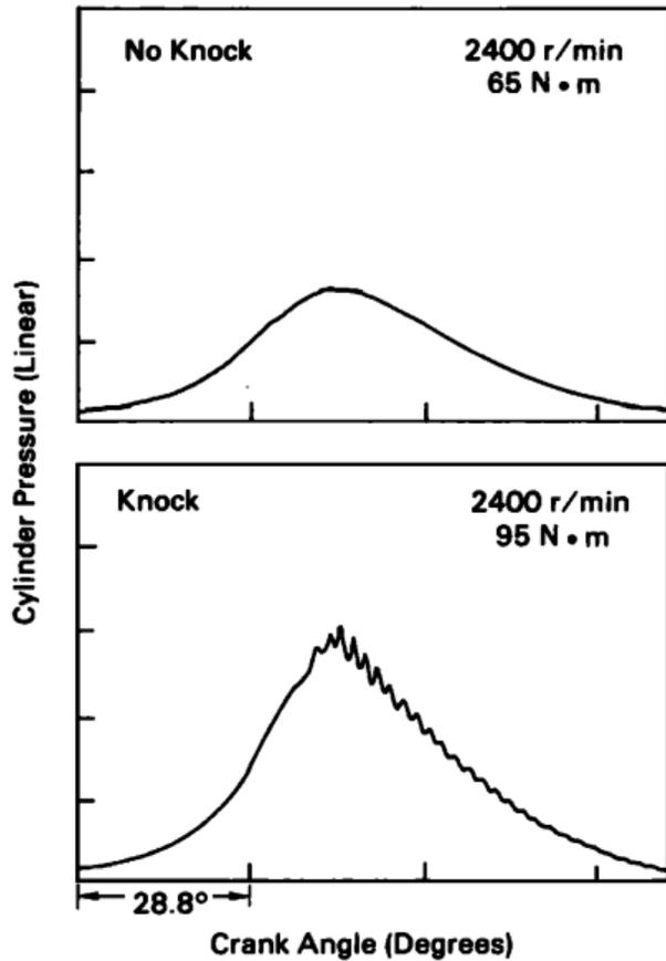
Figure 1. In-cylinder pressure data without (above) and with (below) knock [5], reprinted with permission.
