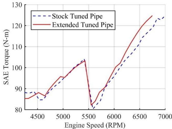
Figure 11. Torque comparison of stock and extended tuned pipes.
