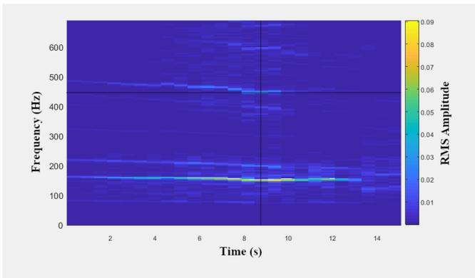
Figure 5. Frequency versus time plot with 2018 track and driver configuration measured on the clutch side. Crosshairs indicate frequency identified as the track and driver interaction.
