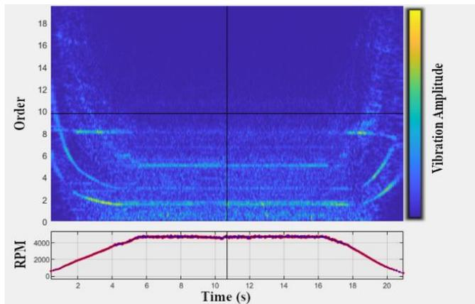
Figure 3. Vibration order with respect to driveshaft RPM.
