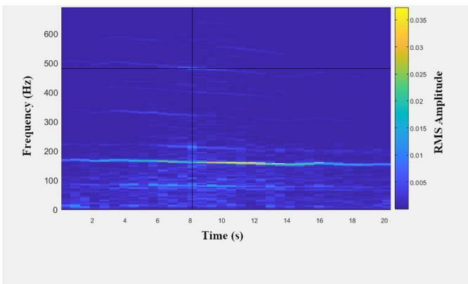
Figure 6. Frequency versus time plot with Silent Track II installed measured on the clutch side. Crosshairs indicate frequency identified as the track and driver interaction.
