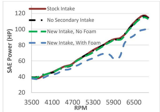
Figure 7. Power sweeps comparing intake configurations.
