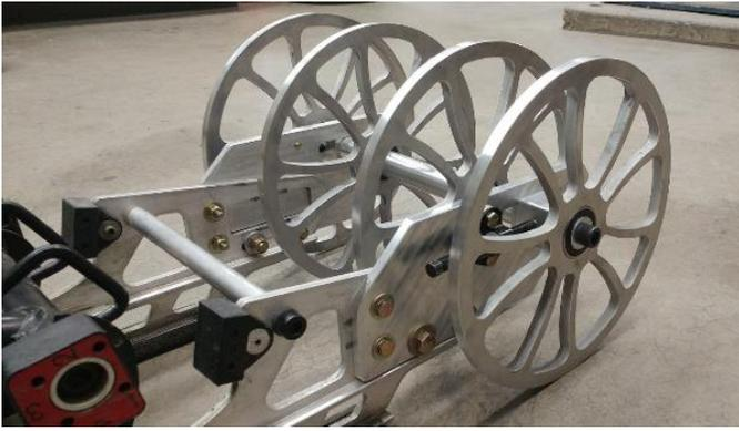
Figure 12. Increased diameter rear idler wheels installed on the skid.
