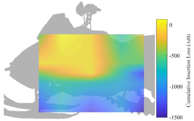
Figure 15. Noise vectoring results from the clutch side of the snowmobile.
