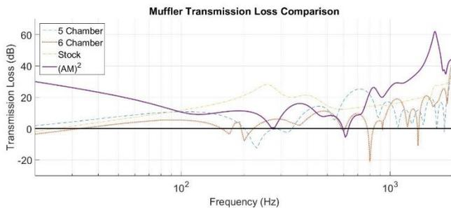
Figure 15. Muffler Sidlab results.
