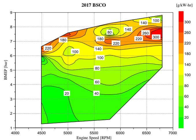
Figure 9. Brake specific CO production.
