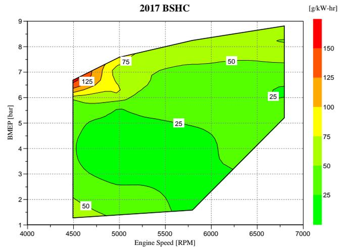
Figure 8. Brake specific UHC production.
