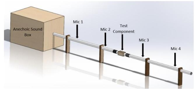
Figure 14. UICSC sound box configuration.
