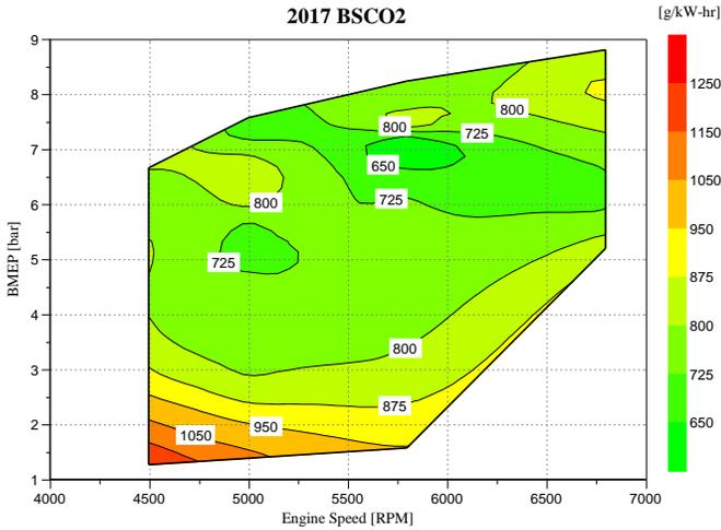
Figure 10. Brake specific CO2 production.
