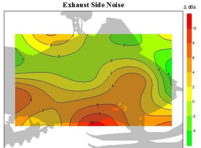
Figure 12. Noise vectoring for exhaust side.
