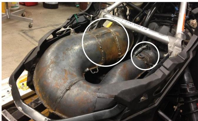
Figure 3. Extended tuned pipe in chassis.
