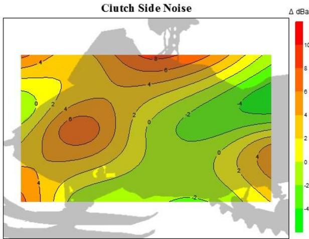
Figure 13. Noise vectoring for clutch side.
