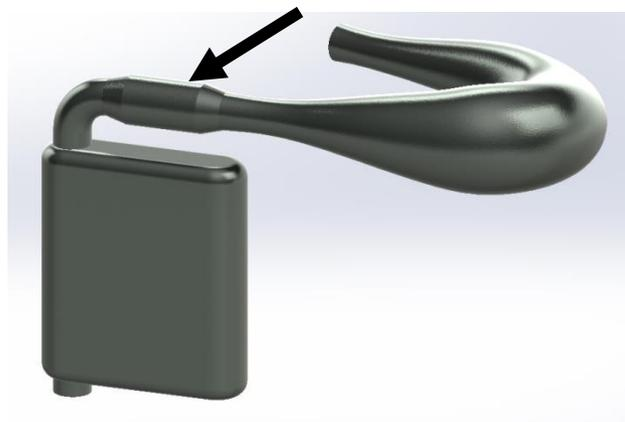
Figure 7. Relocation of catalyst.
