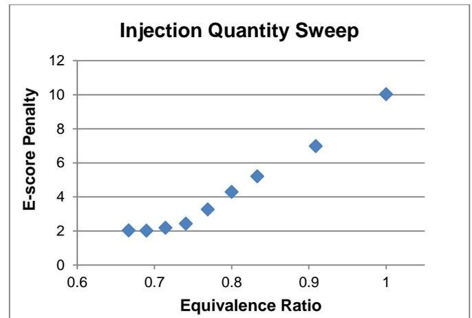
Figure 2: Penalty function vs. equivalence ratio at a constant injection timing.
