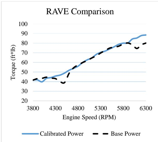
Figure 14: Comparison of power drops accelerating through RAVE openings
