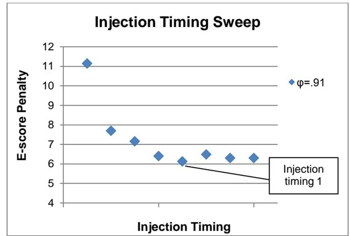
Figure 1: Penalty function vs. injection timing at a constant equivalence ratio.
