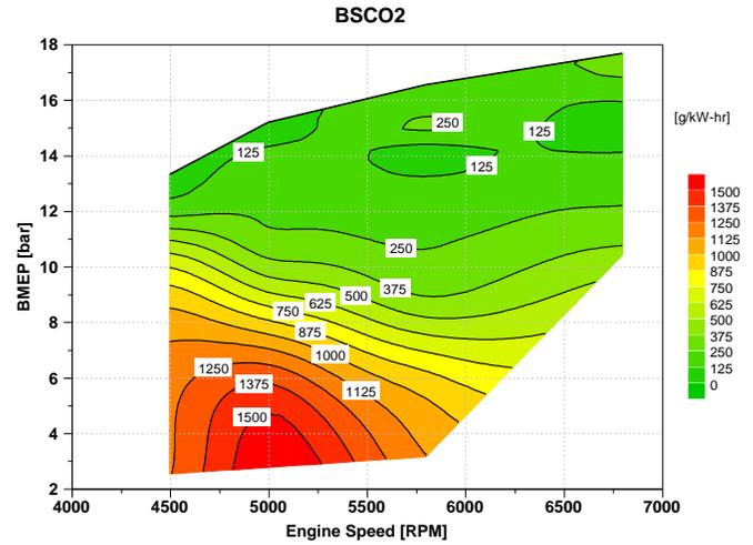
Figure 13: Brake specific CO<sub>2</sub> production
