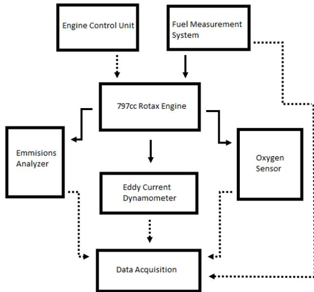
Figure 17: Test equipment data flow.
