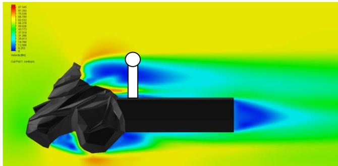
Figure 18: CFD simulation of airflow with windshield
