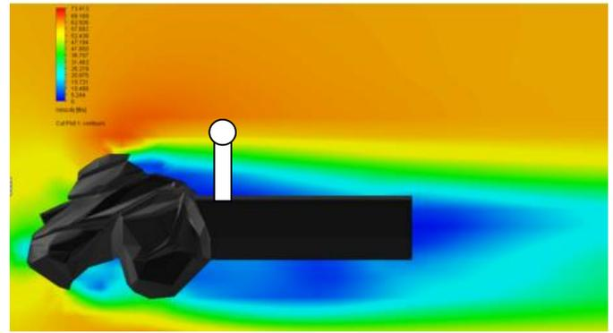
Figure 16: CFD simulation of airflow without windshield.
