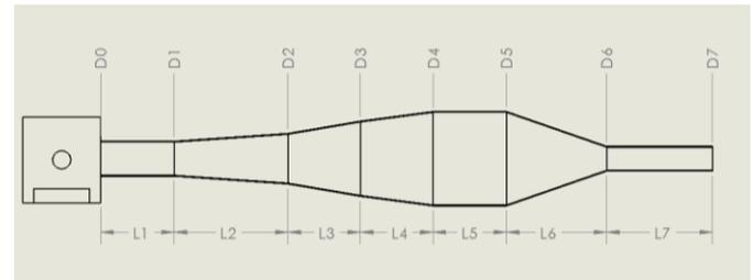
Figure 3: Visual representation of a tuned exhaust
