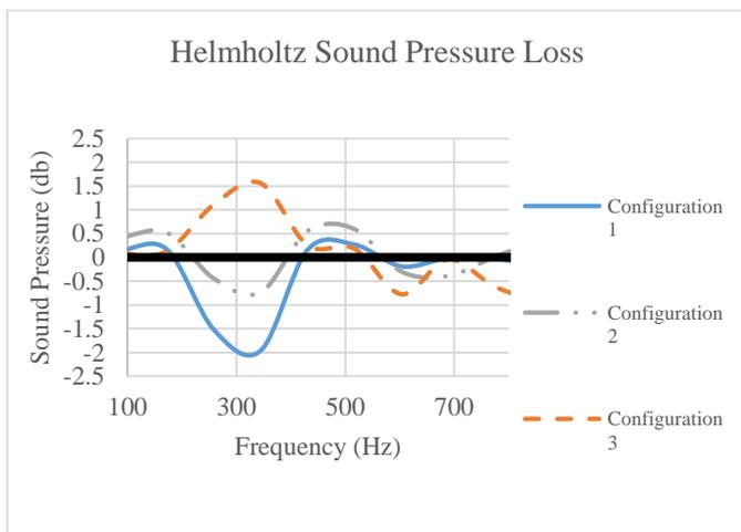
Figure 6: Comparison of various Helmholtz configurations
