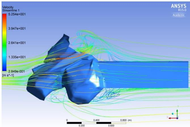
Figure 17: Software simulation showing flow patterns over snowmobile chassis
