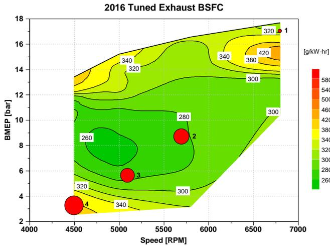
Figure 7: Brake specific fuel consumption map for 2016 exhaust
