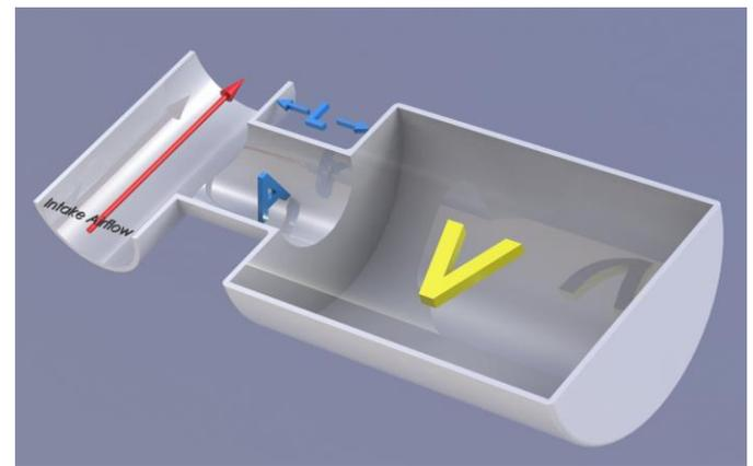
Figure 5: Visual representation of Helmholtz configuration chosen
