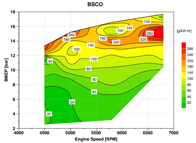
Figure 12: Brake specific CO production
