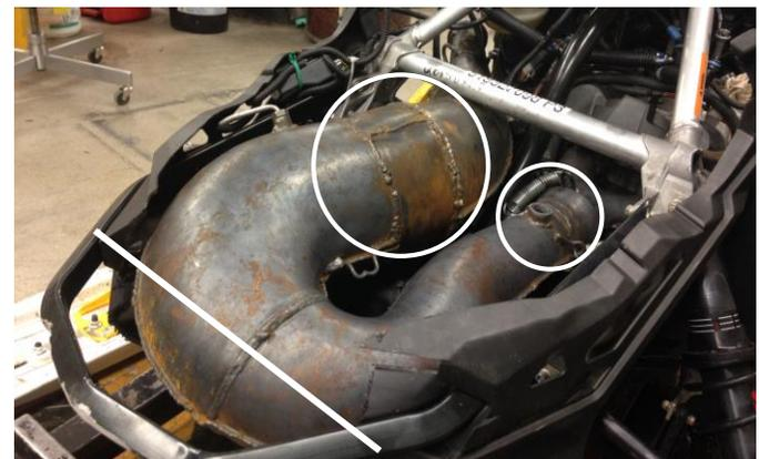
Figure 4: Extended tuned pipe in chassis
