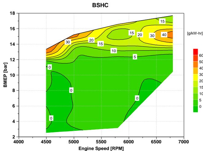
Figure 11: Brake specific UHC production
