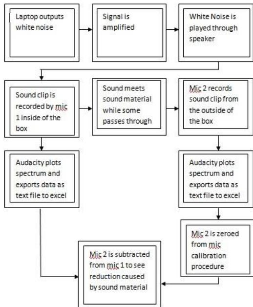
Figure 12. Test setup flow chart
