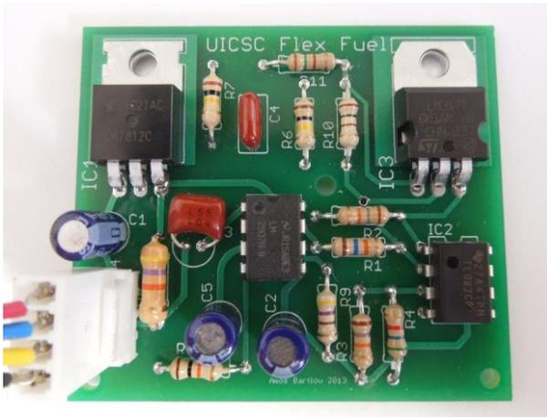
Figure 5. The UICSC printed flex fuel circuit.
