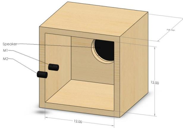
Figure 11. Sound box, materials testing apparatus
