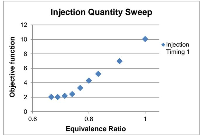
Figure 4. Objective function vs. equivalence ratio at a constant injection timing.
