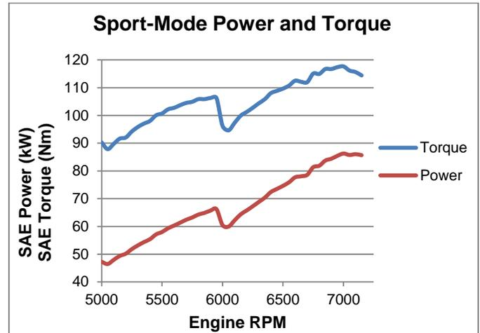
Figure 7. Power sweep for sport-mode (measured horsepower).
