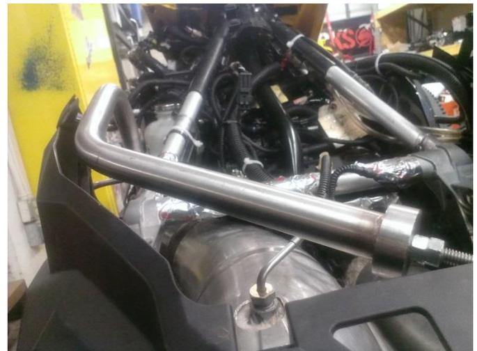
Figure 15. The Quarter wave resonator packaged in chassis.
