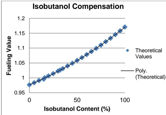
Figure 6. Theoretical and calibrated compensation for blended isobutanol fuels.
