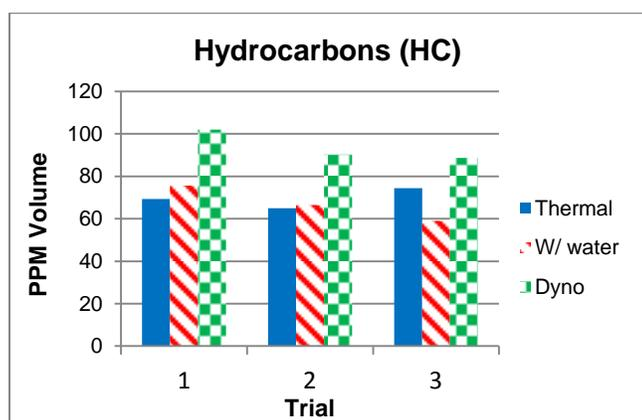
Figure 10. Hydrocarbon emissions after catalyst aging.
