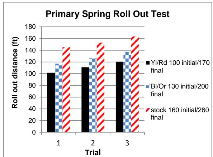
Figure 17. Comparison of three different clutch springs rollout at different speeds
