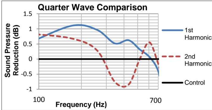
Figure 16. Sound pressure reduced by the 2014 and 2013 quarter wave design in comparison to the stock configuration.
