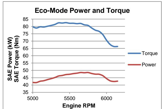
Figure 8. Power sweep for eco-mode (measured horsepower).
