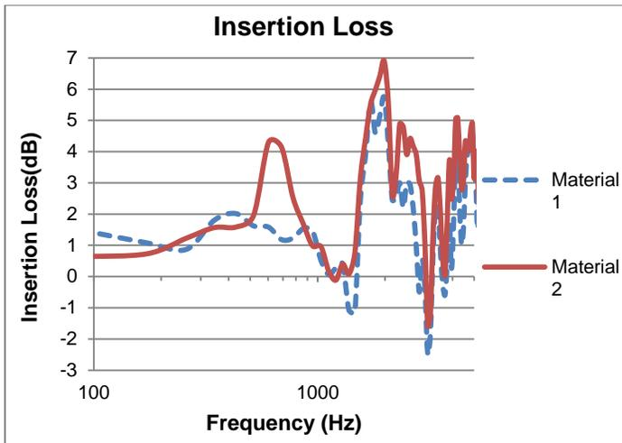
Figure 13. Insertion loss comparison of Material 1 and Material 2.
