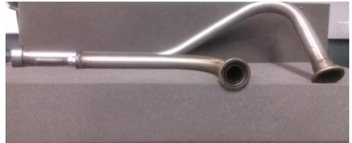
Figure 14. Quarter wave resonator comparison. Previous design in front, new design in the rear.
