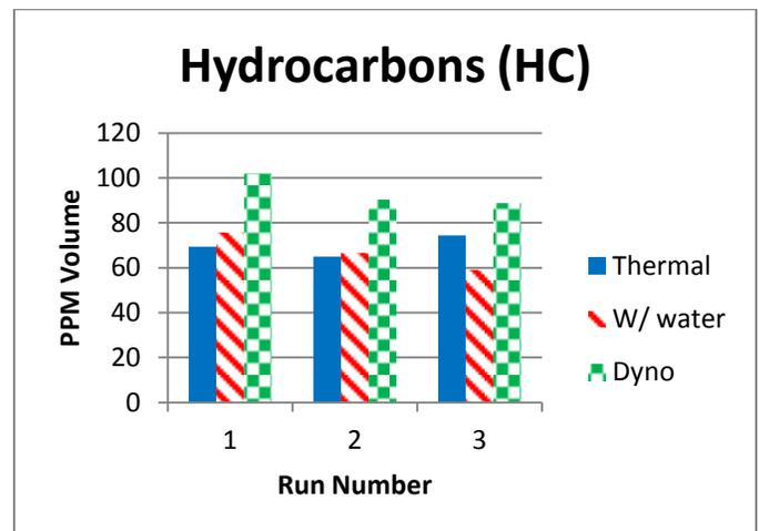
Figure 11: Hydrocarbon emissions after catalyst aging.
