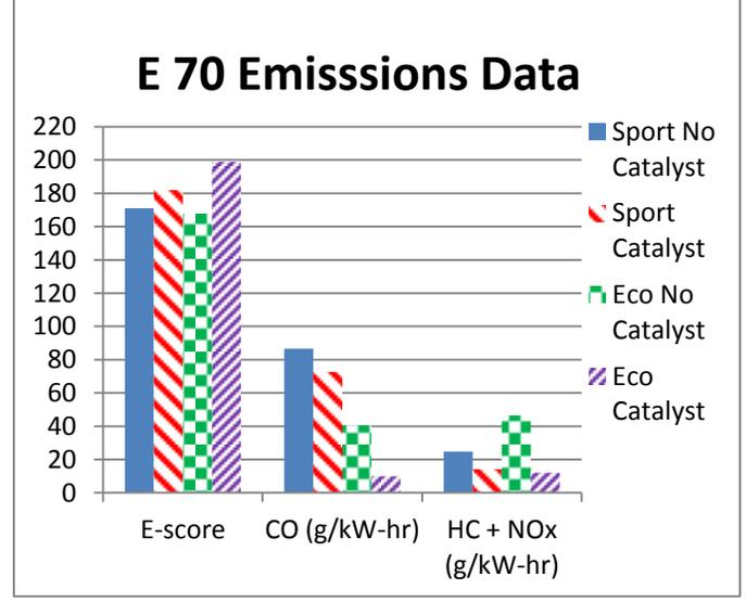
Figure 9: Emissions data for EPA 5 mode tests operating on various ethanol blends.
