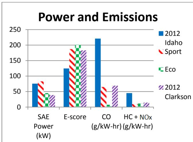
Figure 10: Power and emissions characteristics for different snowmobile configurations.
