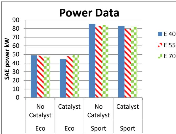
Figure 8: SAE peak power output at two different operating modes.
