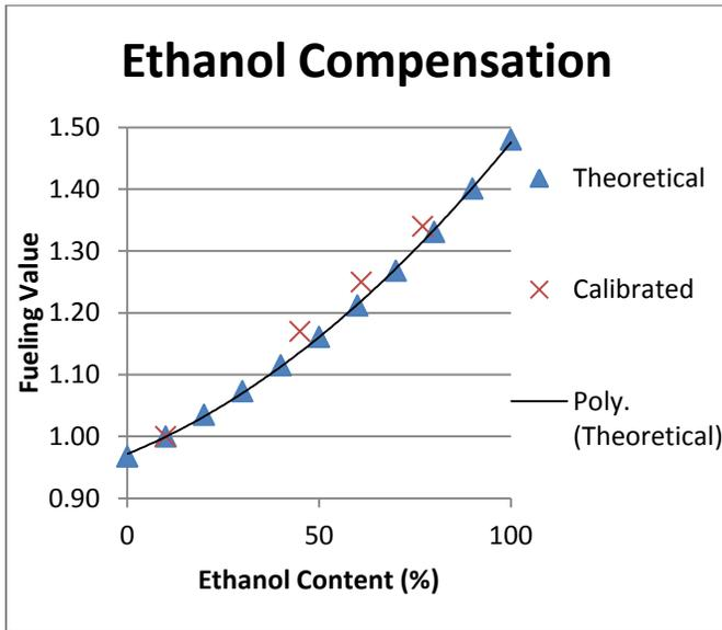
Figure 5: Theoretical and calibrated compensation for blended ethanol fuels.
