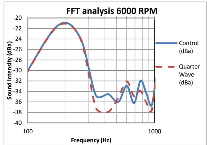
**Figure 13: FFT analysis of UICSC engine operating at a constant speed with and without the quarter wave resonator.**
