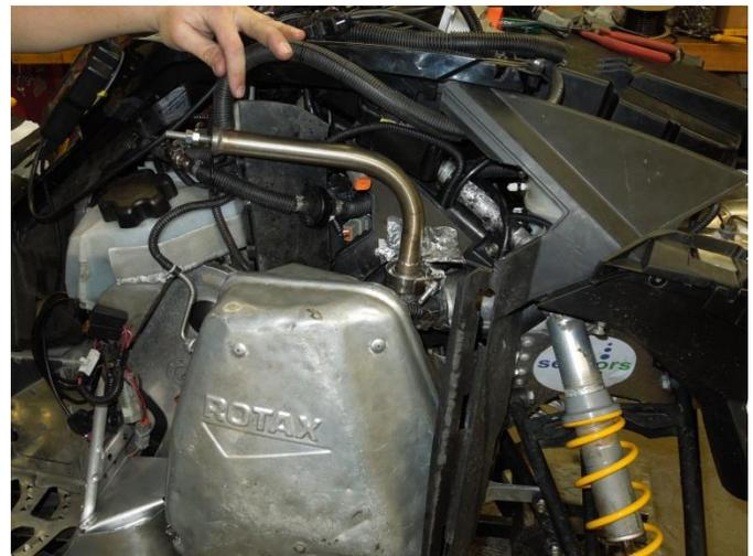
**Figure 14: Quarter wave resonator in chassis.**
