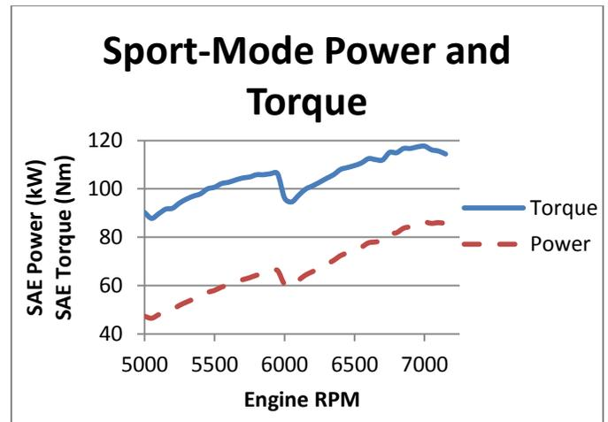
Figure 6: Power sweep for sport-mode (measured horsepower).
