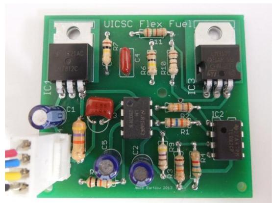
Figure 4: The UICSC printed flex fuel circuit.
