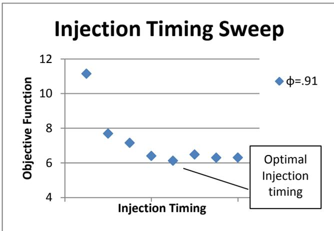
Figure 2: Objective function vs. injection timing at a constant equivalence ratio.
