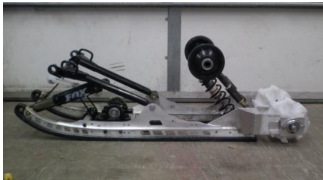
Figure 13 – UICSC rear drive system
