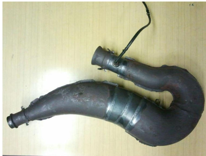
Figure 4 – Completed tune pipe used in the 2012 CSC competition
