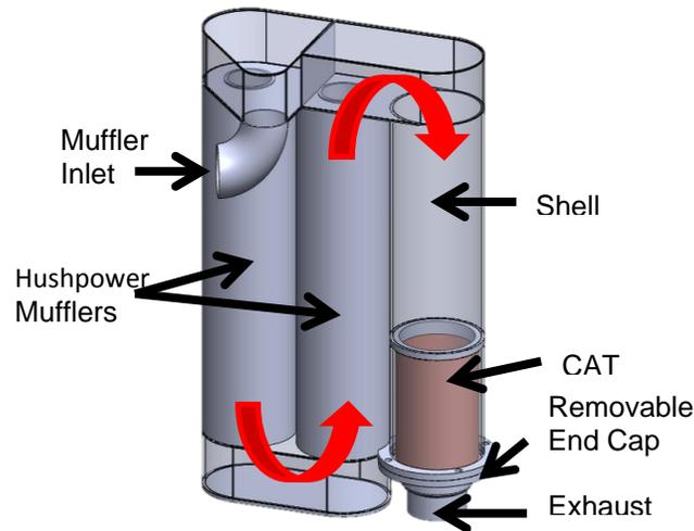
Figure 19: Hushpower and catalyst muffler design.
