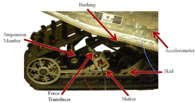
Figure 14: Bushing damper testing layout
