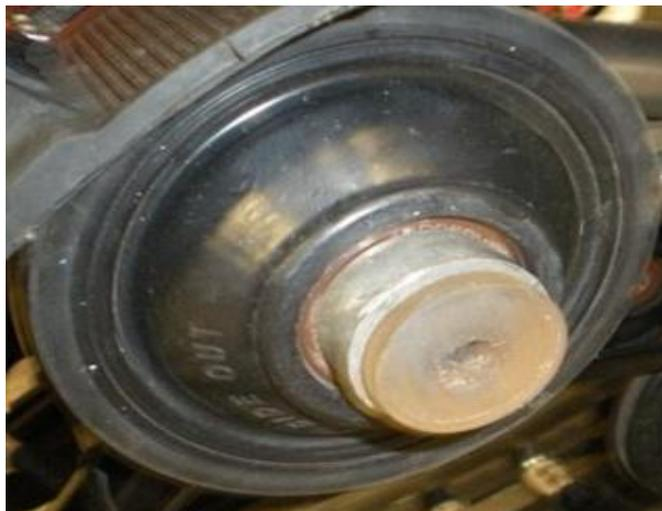
Figure 13: Suspension dampers placed on all connections between track suspension and tunnel.
