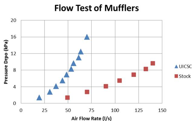
Figure 21: Flow testing results of stock muffler and UICSC muffler.
