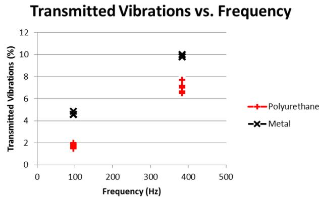
Figure 15: Transmitted vibration percentages through the suspension.
