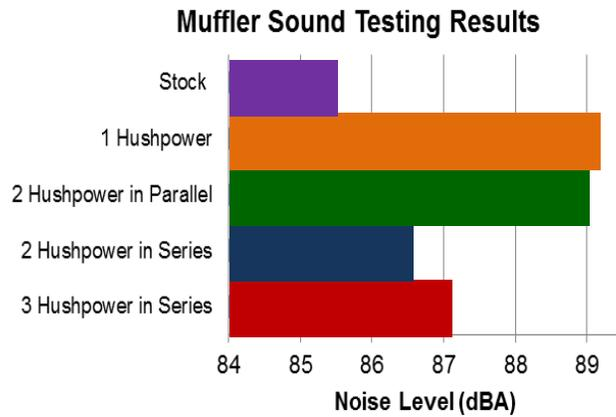
Figure 18: Hushpower muffler configurations vs. stock muffler using J-192 procedures.
