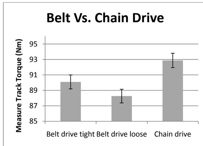
Figure 10: Belt Drive vs. Chain Drive
