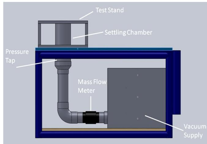
Figure 20: Solid Model of Flow Bench Design
