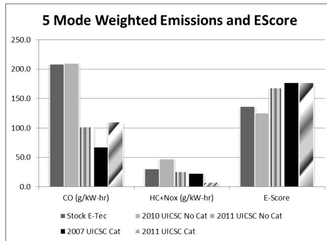
Figure 6 – A 5-Mode weighted emission and E-Score comparison
