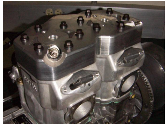
Figure 5: Completed UICSC DI head installed on the Rotax 600 H.O. engine.
