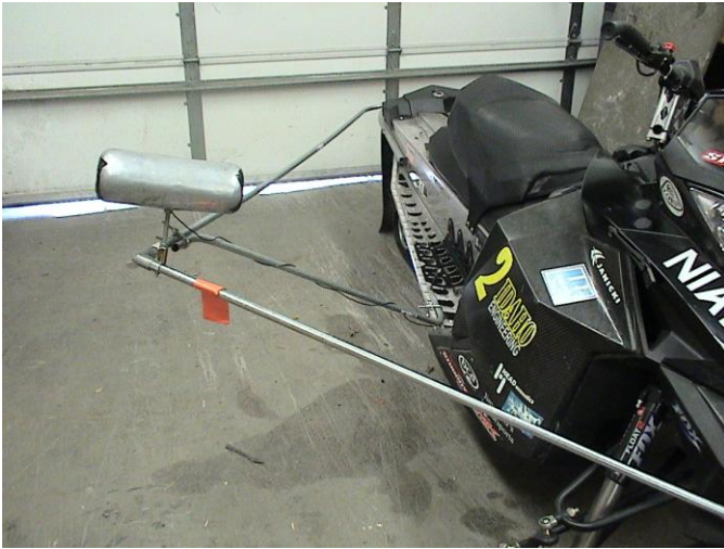
Figure 9: Airfoil and frame to hold Microphone for coherence testing.
