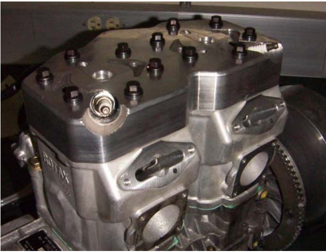
Figure 5: Completed UICSC GDI head installed on the Rotax 600 H.O. engine.
