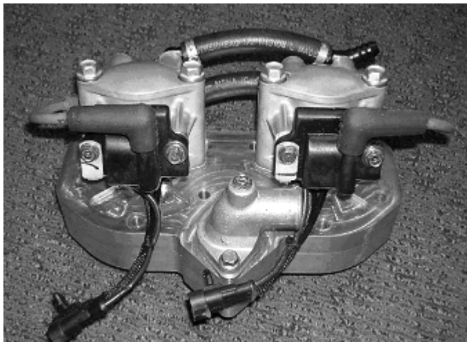
Figure 9: Completed UICSC GDI head with the injector/coil assemblies.
