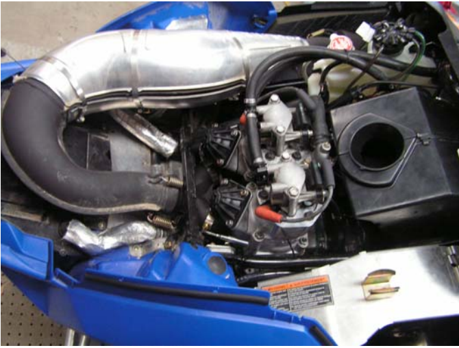
Figure 18: Final design of the UICSC GDI snowmobile.
