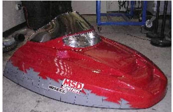
Figure 7: The Lexan™ hood used on the UICSC snowmobile.
