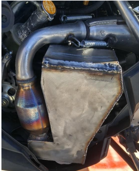
Figure 8 Previous Student-Built Design with Chosen Catalytic Converter
