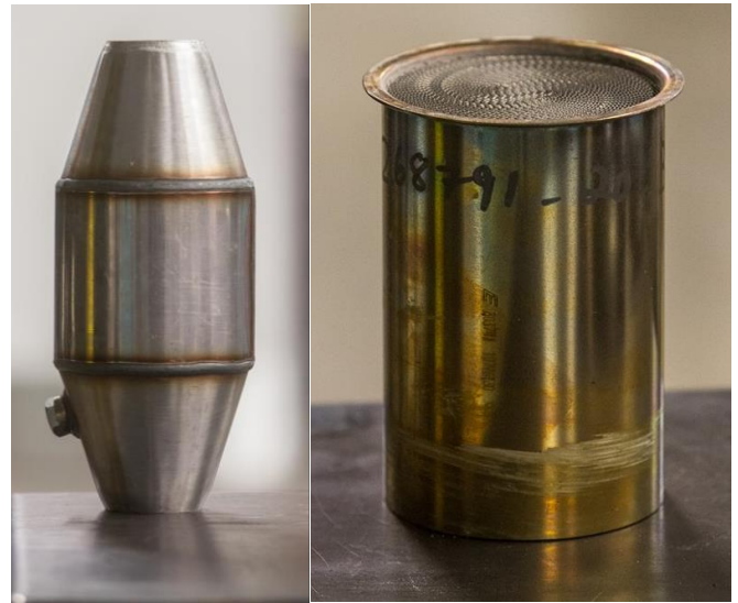
Figure 9. DPF and DOC Used with our Kohler Engine
