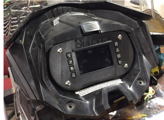
Figure 17. Murphy HV450 Display in our Custom Enclosure
