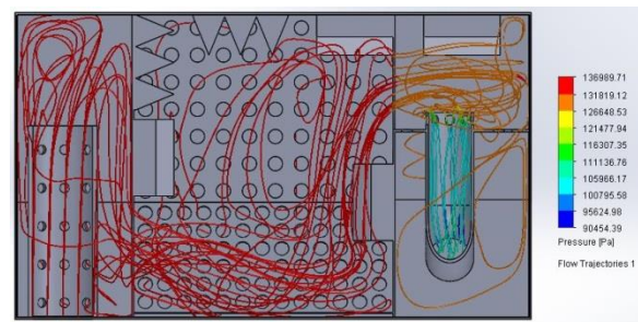
Figure 15. SolidWorks flow simulation. Exhaust enters in the red section, and the pressure drops throughout to the blue.
