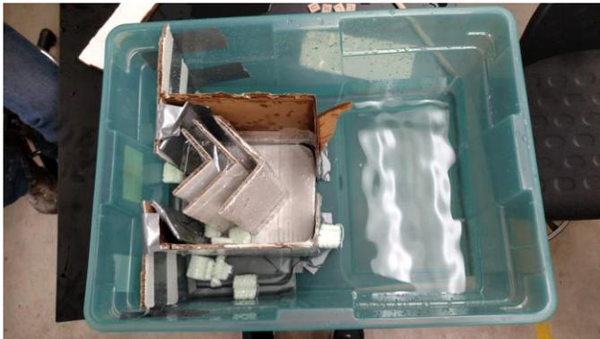
Figure 11. Model of internal baffles used for water testing.
