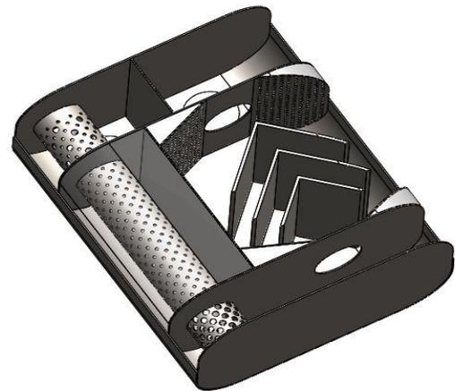
Figure 10. SolidWorks rendering of the muffler
