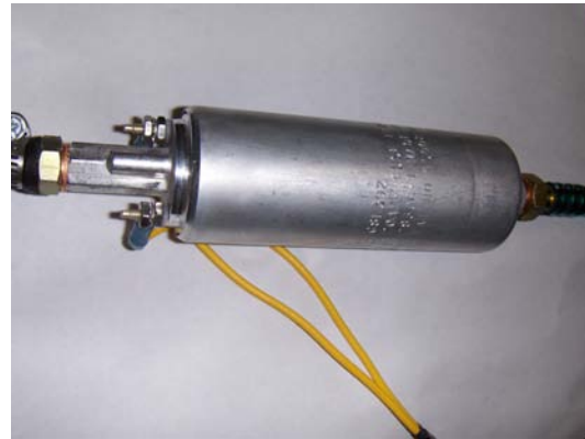
Figure 2: E85 Compatible Fuel Pump
