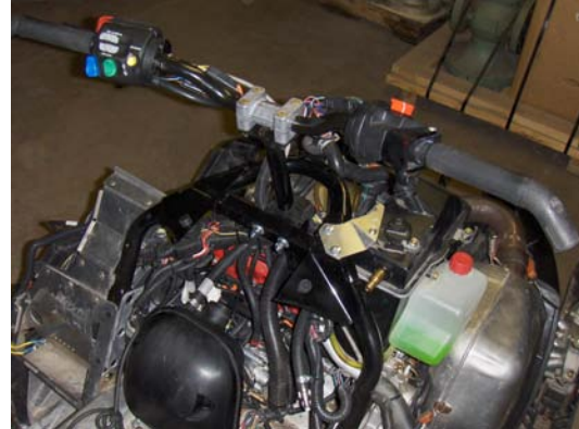
Figure 12: Modified steering post support which encourages rider forward seating.
