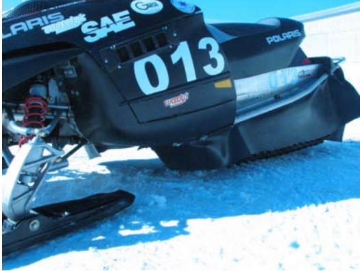
Figure 11: Rubber track and chassis noise dampening skirt.
