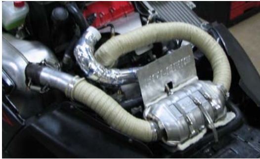
Figure 6: Exhaust system configuration with catalytic converter
