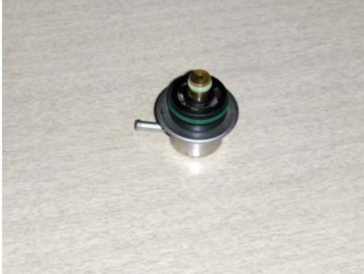
Figure 3: 4.00 bar Fuel Pressure Regulator
