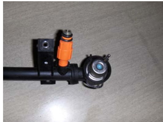
Figure 4: Fuel Injector on Pressure Regulator on Fuel Rail
