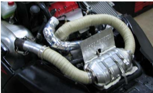
Figure 1: Mount of Catalytic Converter and Exhaust Pipe Routing
