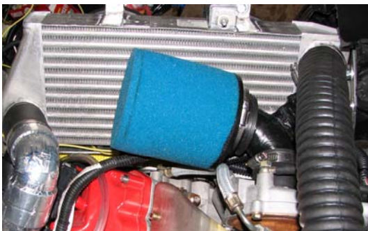
Figure 3: Right Hand View of Intercooler and Intake Air Filter
