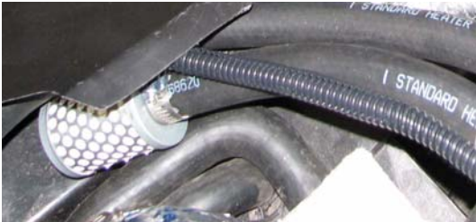
Figure 5: Air Intake Filter for Forced Air Pump
