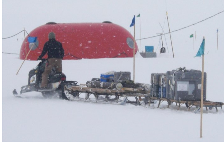
Figure 12 - Electric Snowmobile Towing Research Equipment in Greenland (Photo Courtesy of Scott Keefe)
