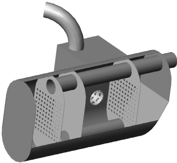
Figure 1: Cut-away view of muffler.
