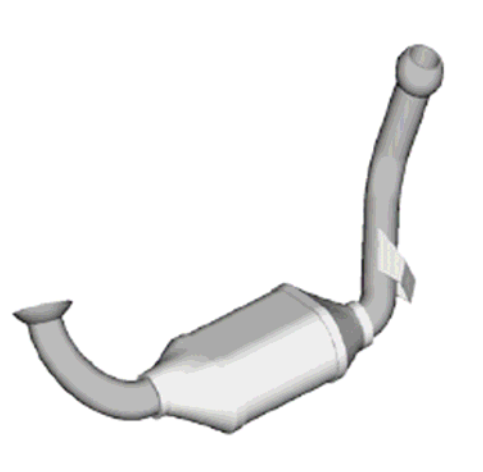
Figure 4: Catalytic converter and exhaust down tube.
