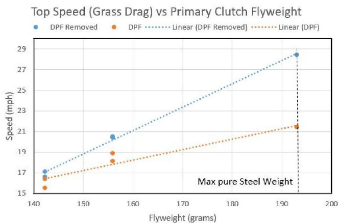
Figure 14. Vehicle top speed utilizing 143g, 156g, and 193g flyweights.
