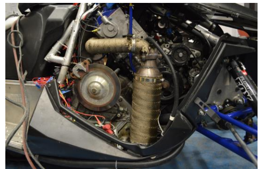
Figure 5: Catalyst and Diesel Particulate Filter
