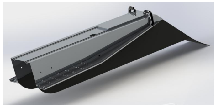
Figure 14. SolidWorks Solid Model of Snow Flap Design
