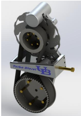
Figure 11. Belt Drive Assembly Designed in SolidWorks
