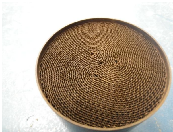
FIGURE 1: Picture of an EMITEC partial flow DPF
