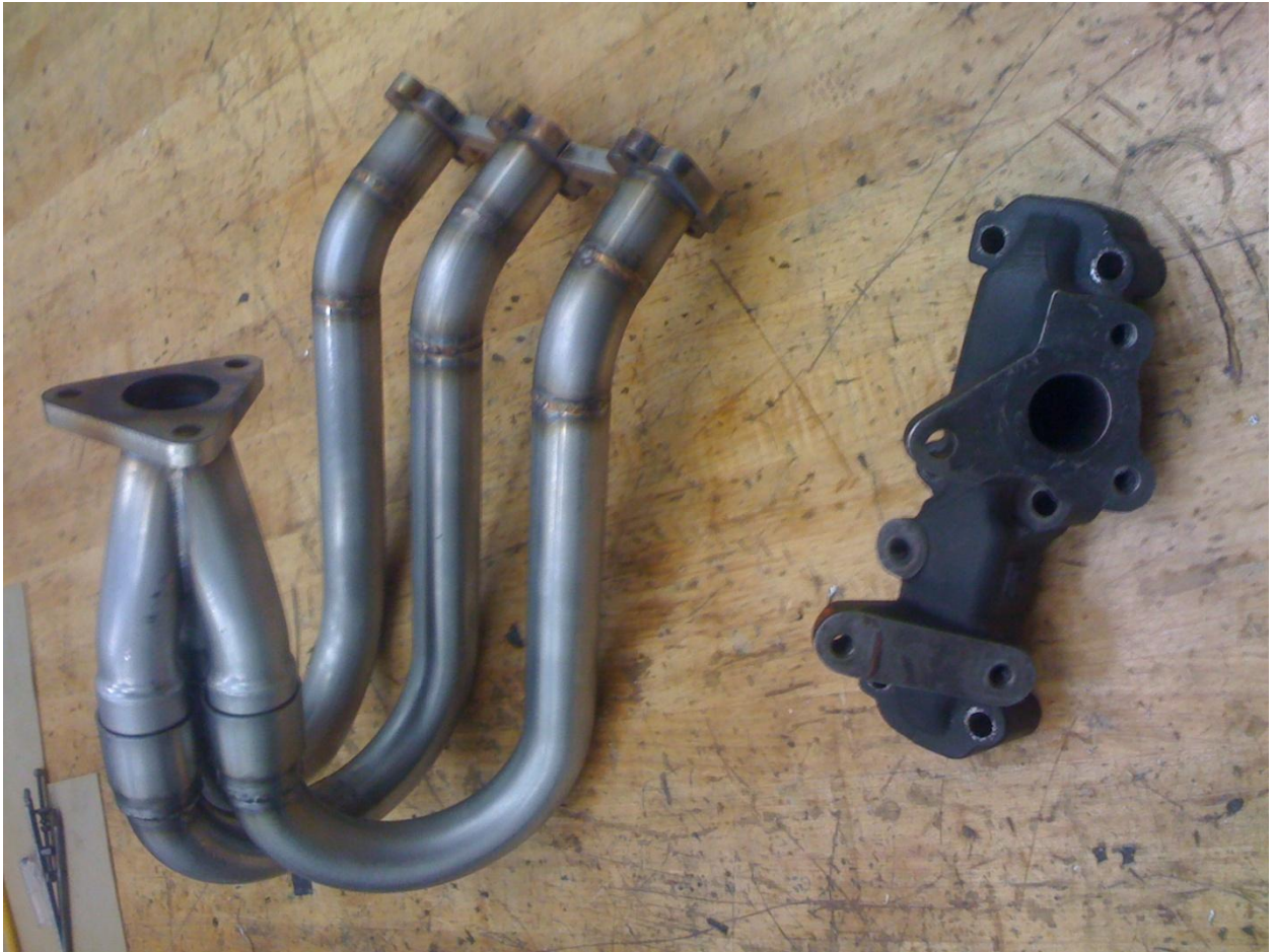
APPENDIX FIGURE 4: Actual picture of old and new exhaust manifolds
