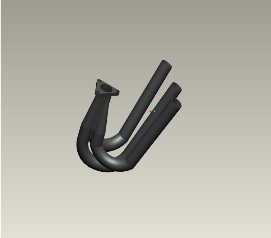
APPENDIX FIGURE 3: Solid model of exhaust manifold
