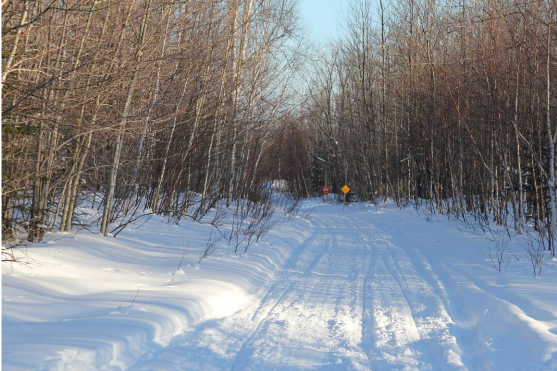
Figure 32 View of worded stop ahead on high speed section of trail. Placement of warning sign was 85 feet from stop sign (see section 4.2.1 for an explanation of this distance).
