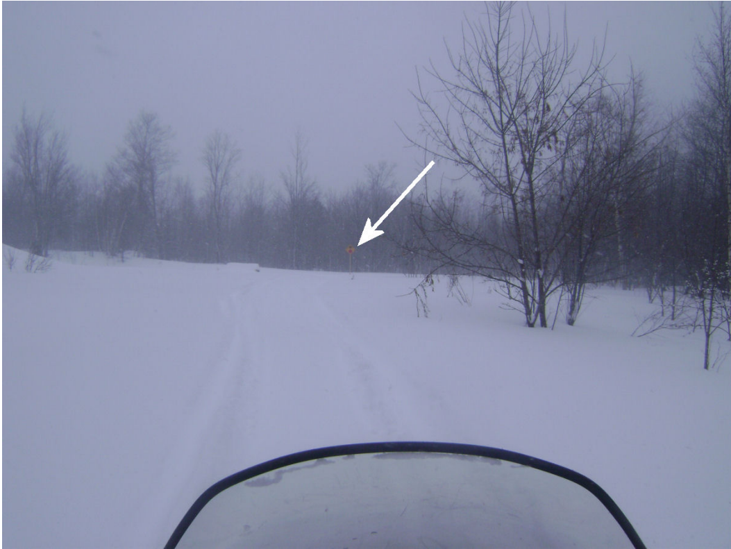
Figure 21 Photograph of a symbol stop ahead sign from a distance of 425 feet.
