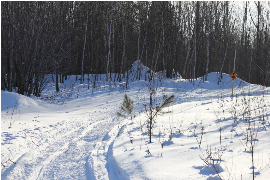
Figure 37 View of 12-inch symbol stop ahead sign placed 126 feet from stop sign, before a curve.
