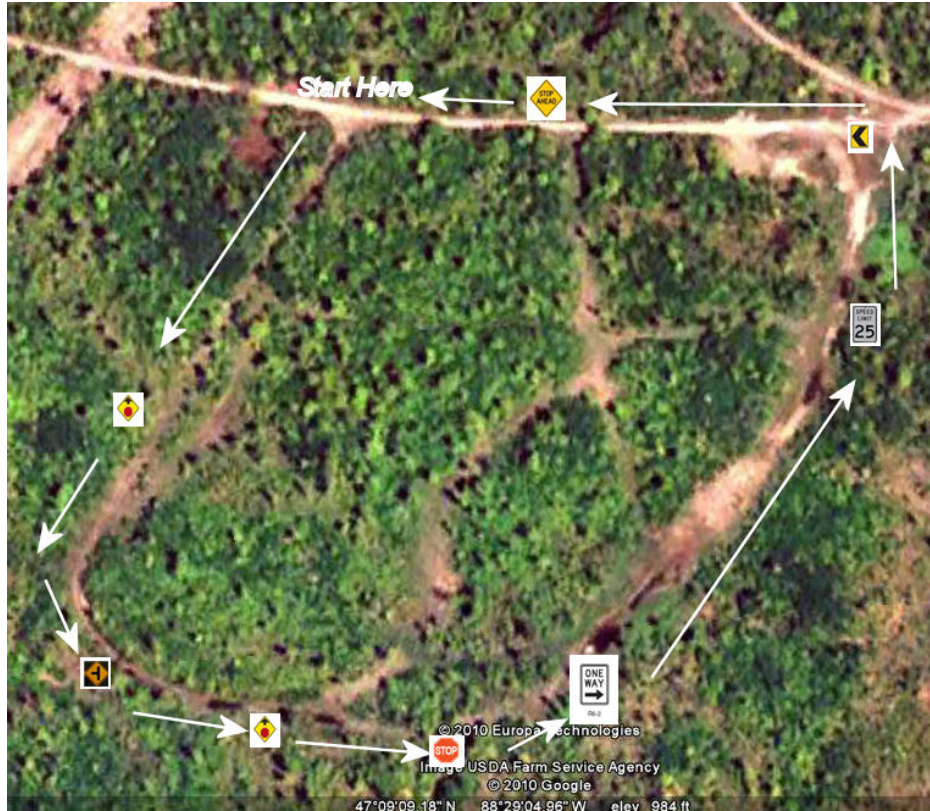
Figure 22 Snowmobile sign recognition sign placement trail layout.
