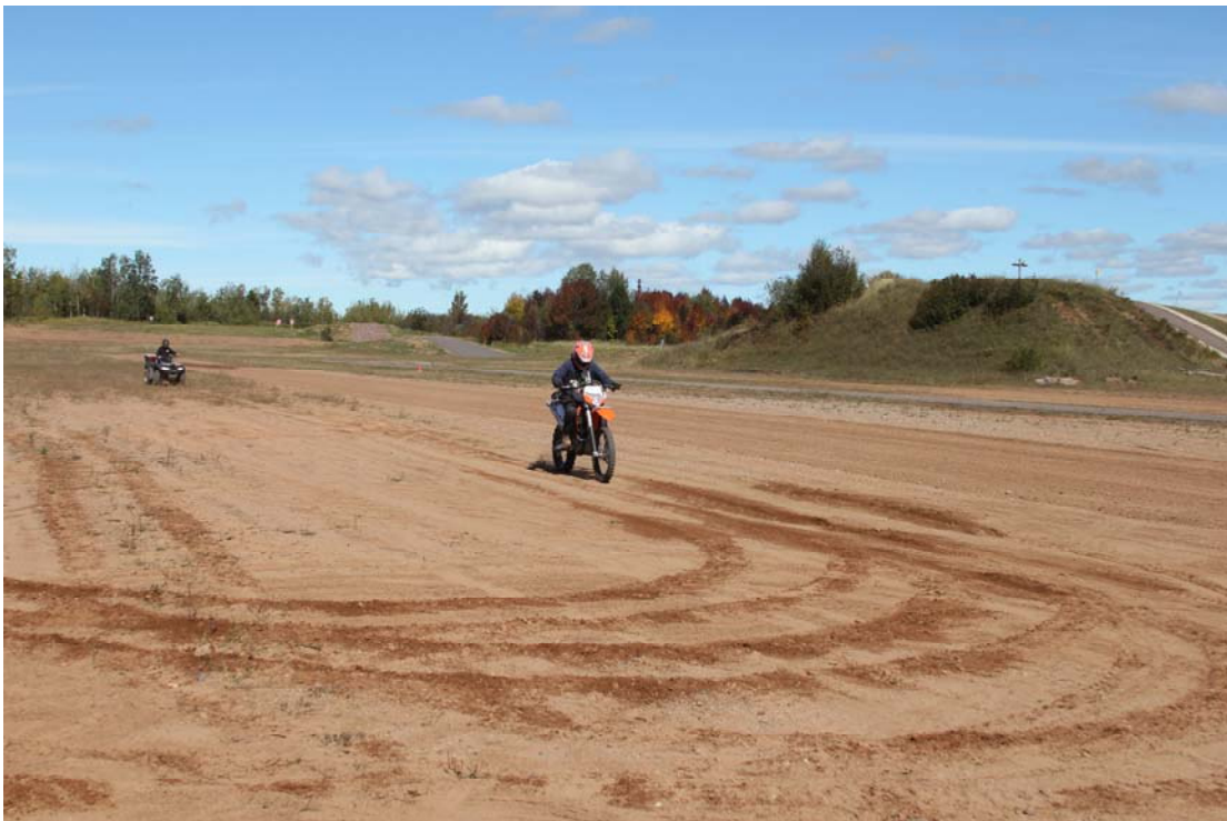
Figure 8 Photograph of the motorcycle braking on flat sandy loam.
