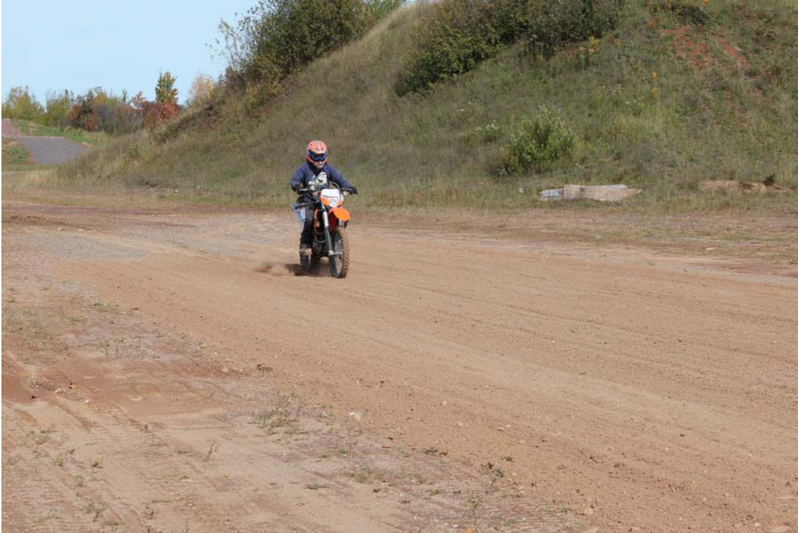
Figure 13 Photograph of motorcycle braking in flat loose sand.
