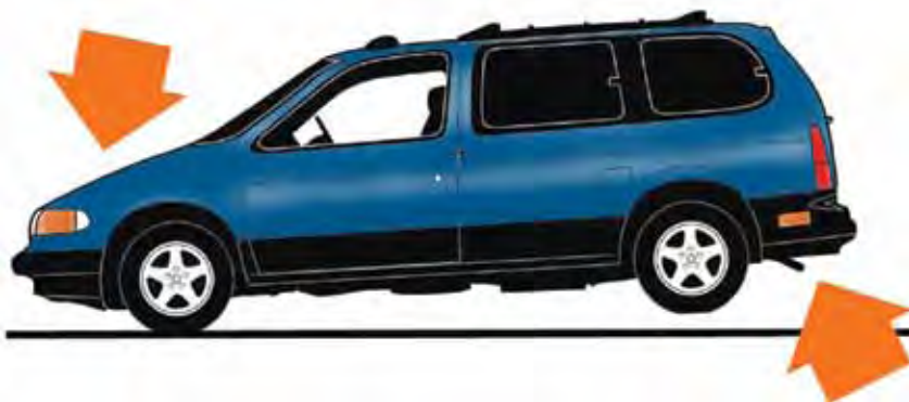
Figure 3. Illustration of weight transfer under acceleration and deceleration
